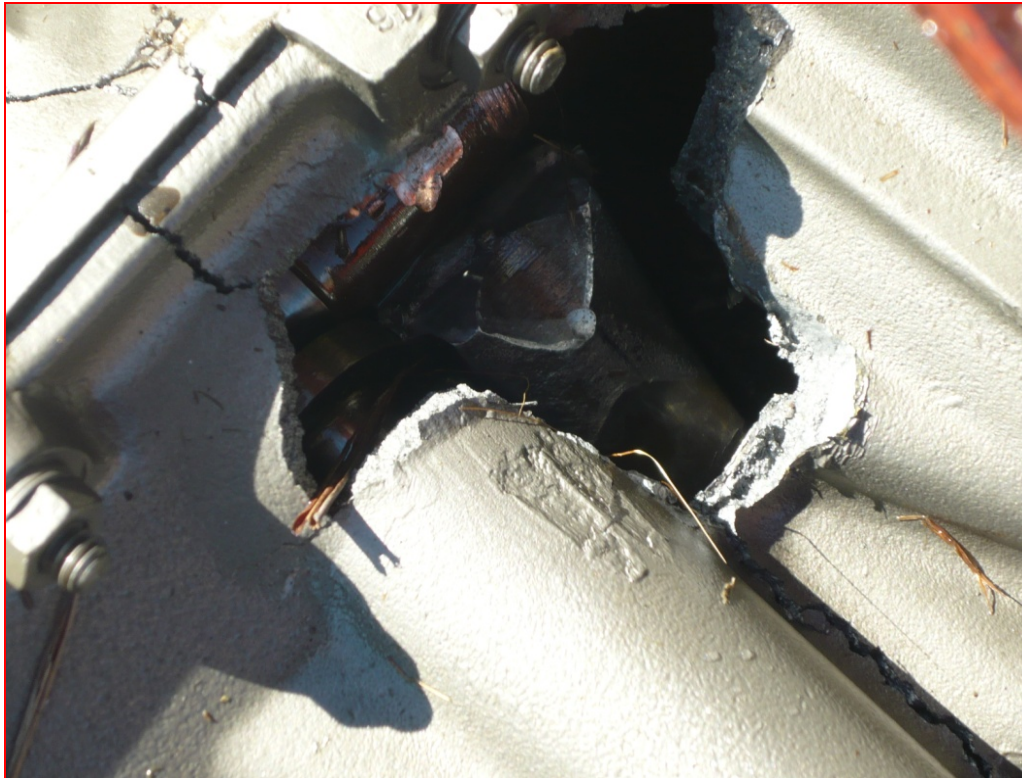
Figure 2. Damage to engine crankcase after failure of conrod attachment bolt.
