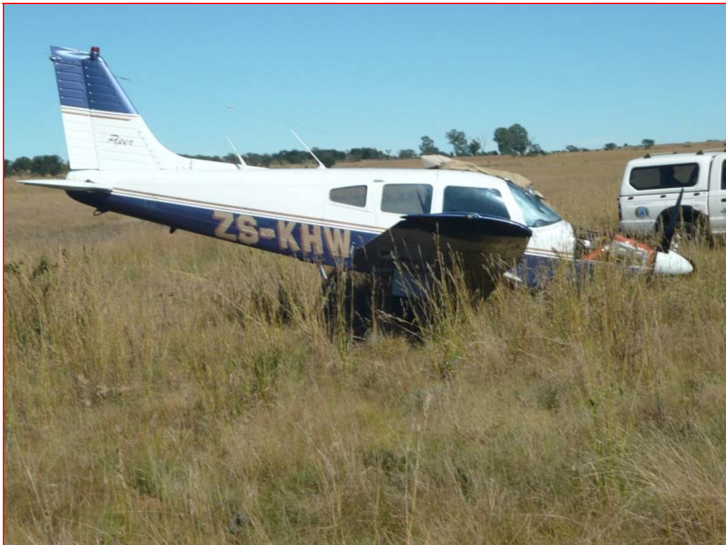
Figure 1. Damage was limited to the nose gear and propeller.
