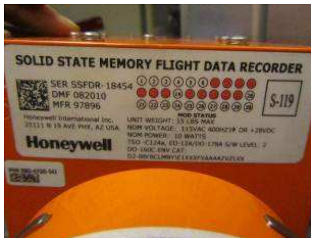
Figure 7: Flight data recorder (FDR) recovered from the aircraft
