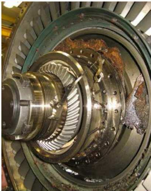
Front view of HPC with IGB bevel gear, locking nut and bearing still sited on HPC shaft
