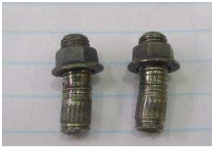
Figure 13: The loose studs with nuts attached found in the engine
