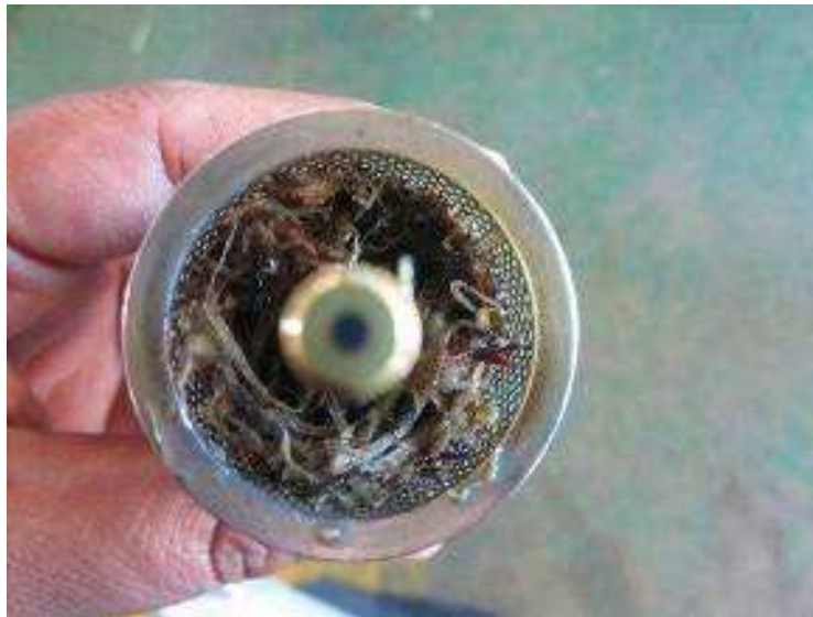
Figure 12: Contaminated forward sump scavenge strainer plug
