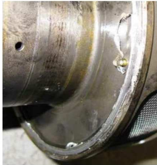
Air-Oil separator with wear
