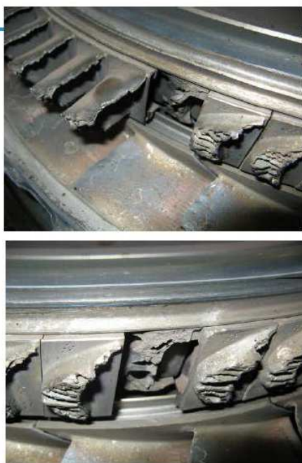
Figure 1. Overviews of ESN890-816 HPT rotor assembly after removal from the event engine. Three HPT blades (two of them shown in the pictures above) had under platform separation. The remaining HPT blade set had missing/broken airfoil above platform as a result of secondary impact damage.
