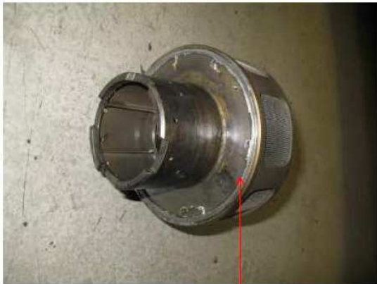
Air-Oil separator with wear
