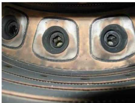
Combustor case in good condition
