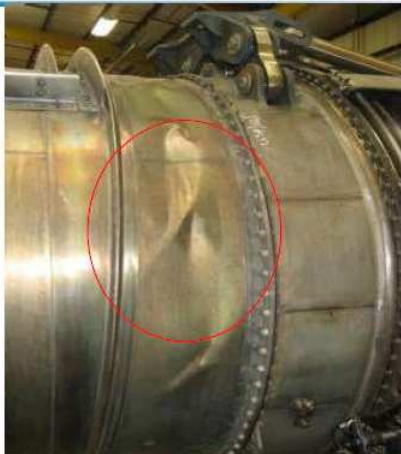
Debris outside the LPT in tailpipe.
