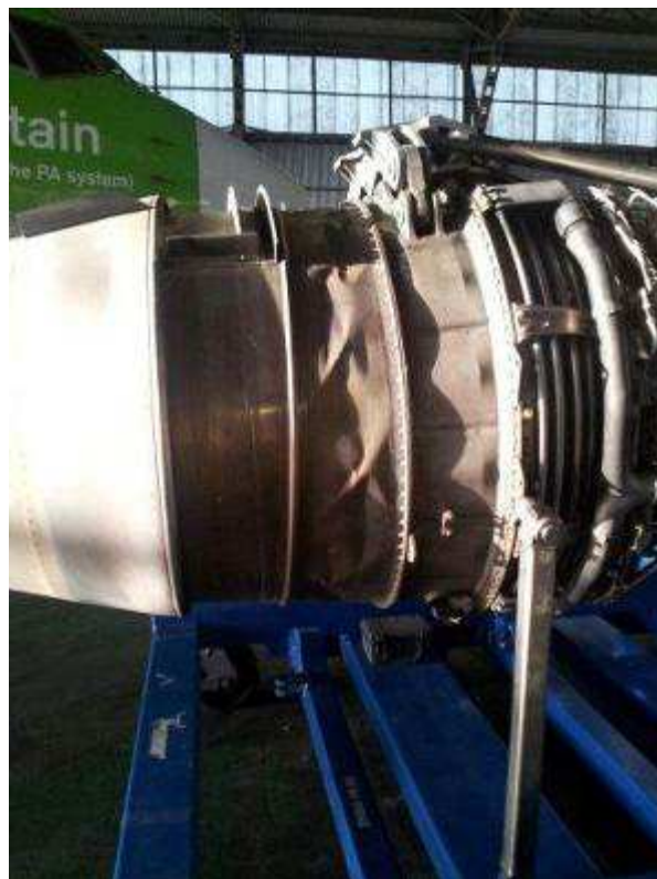
Figure 10: Deformed engine casing
