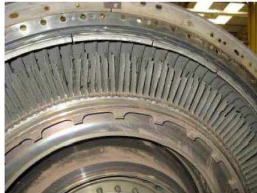
All LPT blades damaged – mostly close to blade tip
