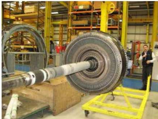
All LPT blades damaged – mostly close to blade tip
