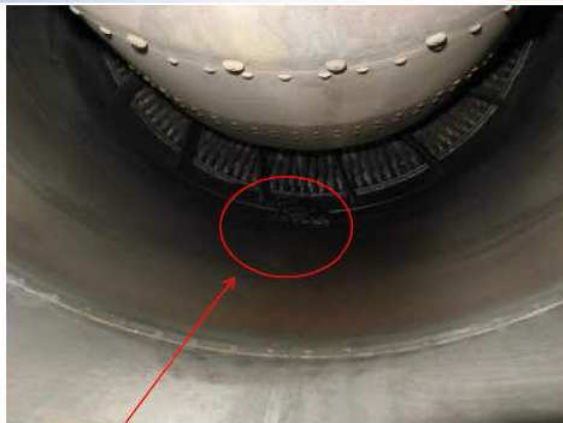
Debris outside the LPT in tailpipe.
