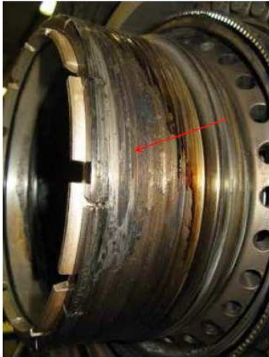
HPT shaft – wear on 3 o'clock position ALF
