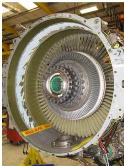
Booster in general good condition. Abradable damage visible after blades removal
