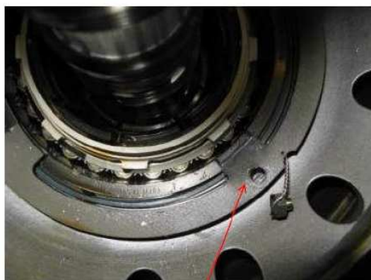
Deformation of #5 bearing retainer ring – one bolt sheared
