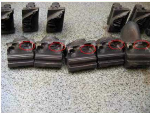
HPT blades with pre-existing cracks under the platform
