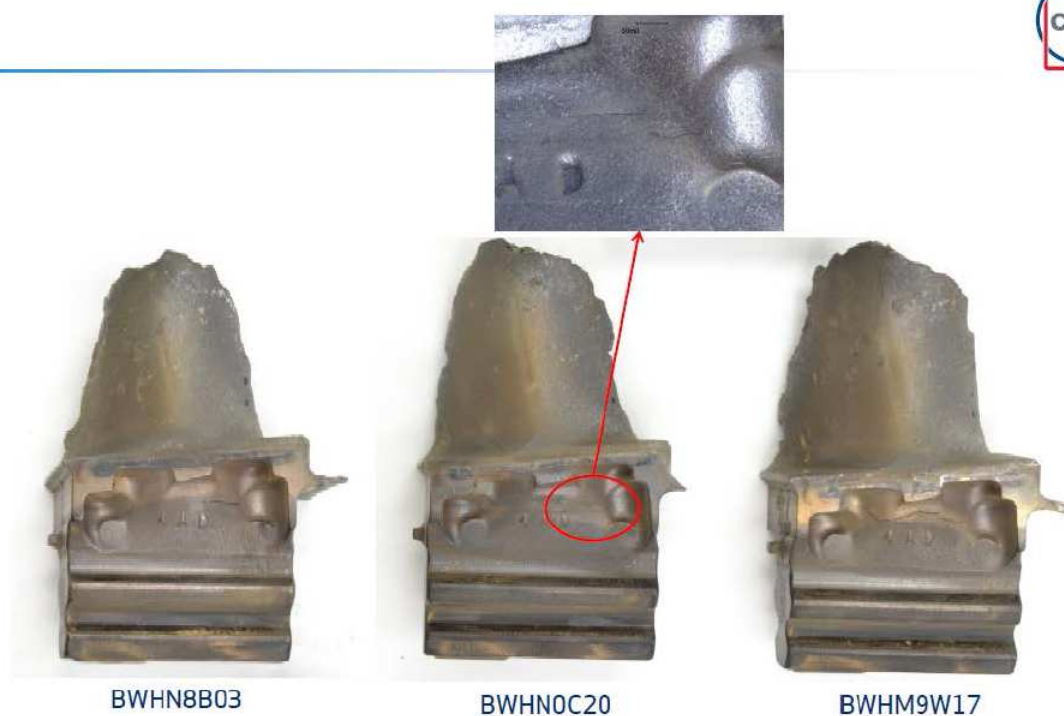
Figure 12. Macro photos showing additional M10P03 blades with visible thru wall transition zone cracks on CVX walls (S/N's BWHN8B03, BWHN0C20, and BWHM9W17).
