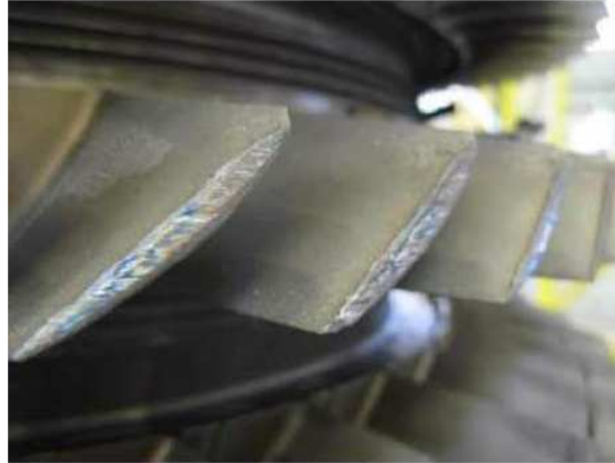
HPC blades with tip wear
