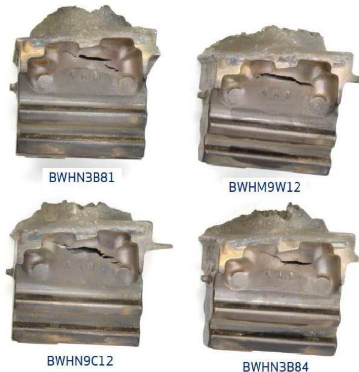
Figure 10. Macro photos showing additional M10P03 blades with visible thru wall transition zone cracks on CVX walls (S/N's BWHN3B81, BWHM9W12, BWHN9C12, and BWHN3B84).
