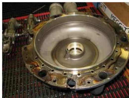
Silver seal on Oil inlet cover with wear
