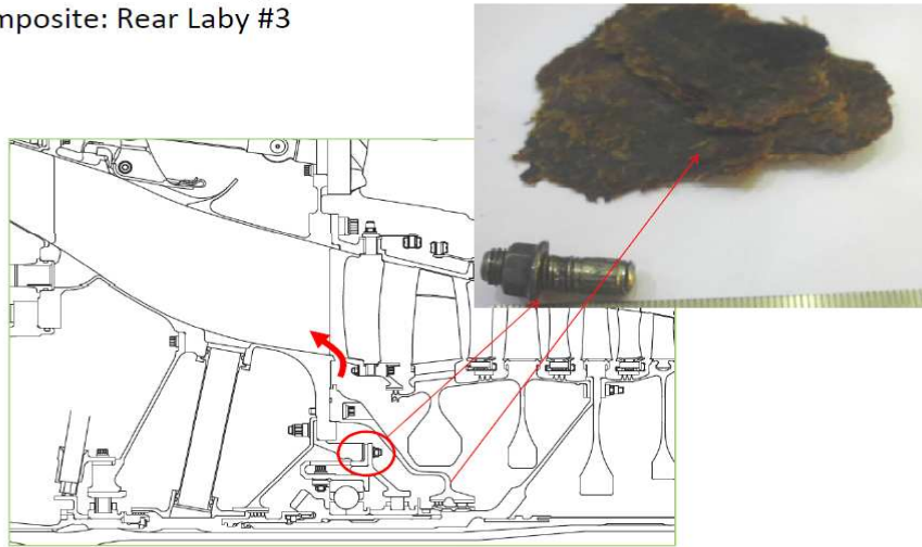
Figure 16: Schematic diagram showing the location of the stud and nut and seal.
