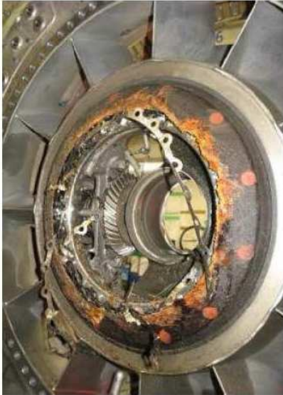
No 3 bearing rear stationary seal separated
