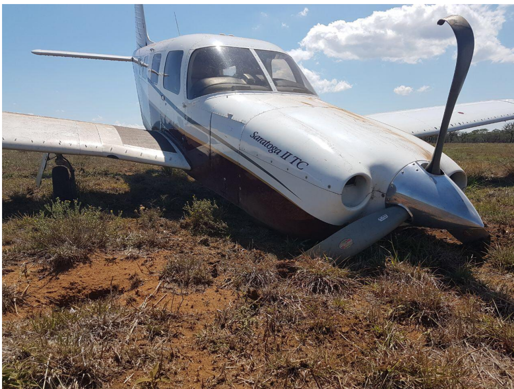
Figure 2: Damage to the propeller
