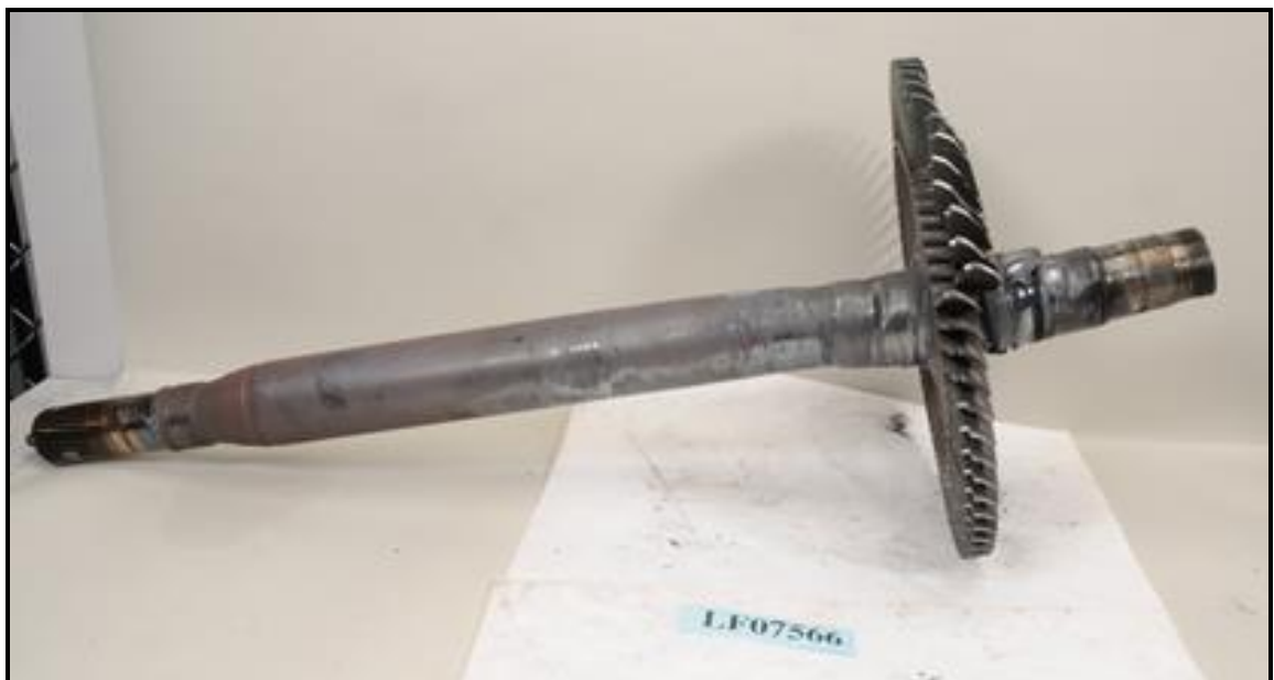
Figure 11: Damages to the LP turbine shaft (deformation)
