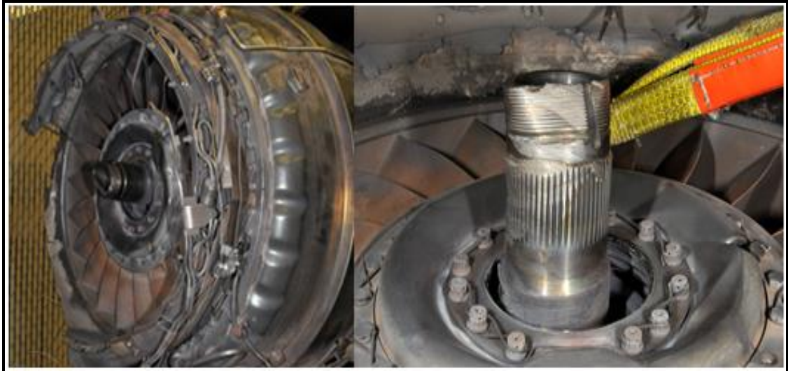
Figure 9: Damage to the drive shaft and the third stator assembly
