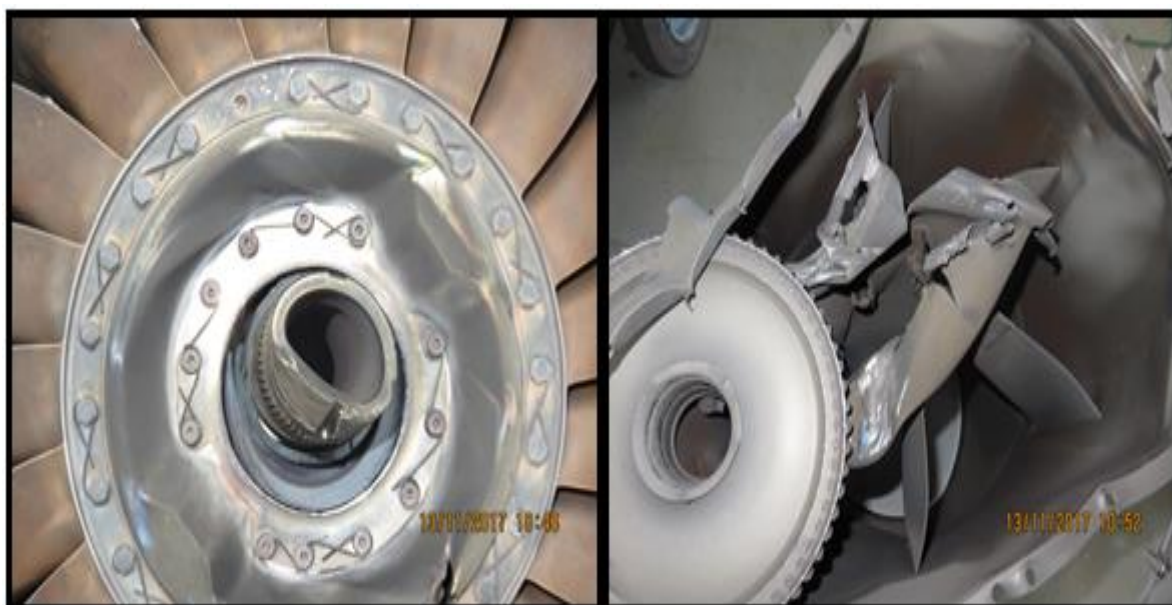
Figure 7: Damage to the shaft assembly and the fourth-stage turbine wheel, as it was found
