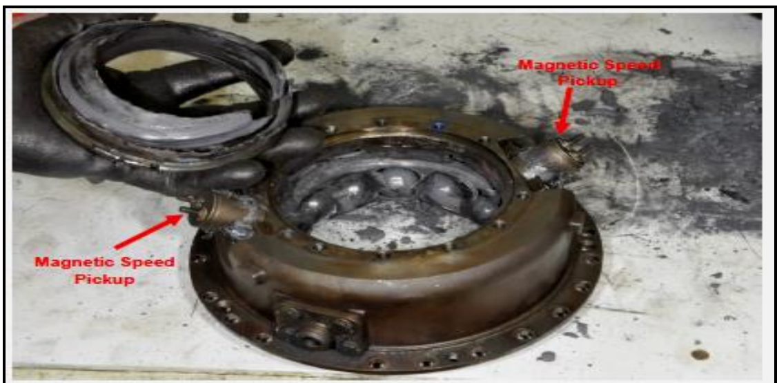
Figure 10: Magnetic over-speed pick-up on the damaged bearing no. 4
