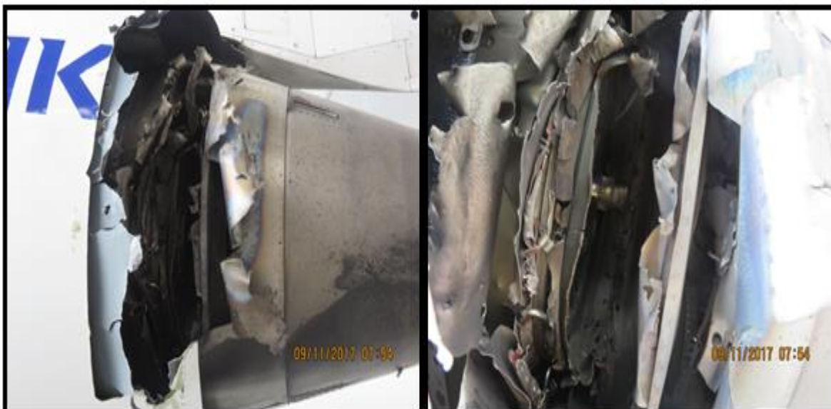
Figure 6: Damage to no. 2 engine's fourth-stage turbine casing
