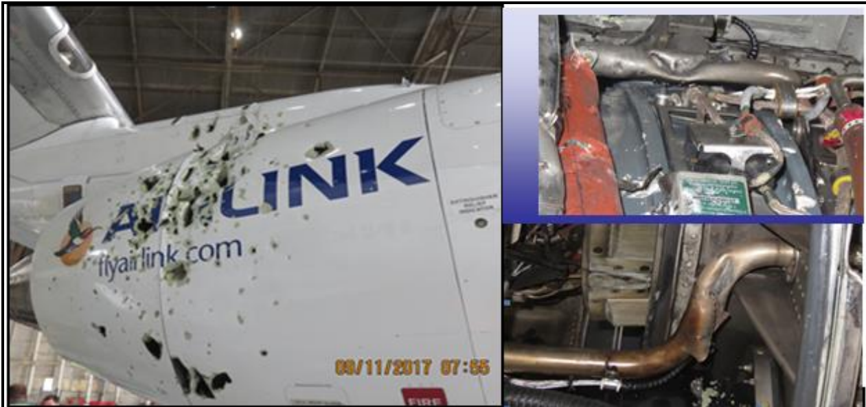
Figure 8: Damage to the engine cowlings, fuel and pneumatic lines, and FADEC box from engine no. 1
