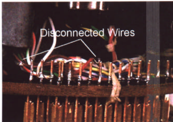
Figure 3: C-14A Directional Gyroscope showing disconnected wires
