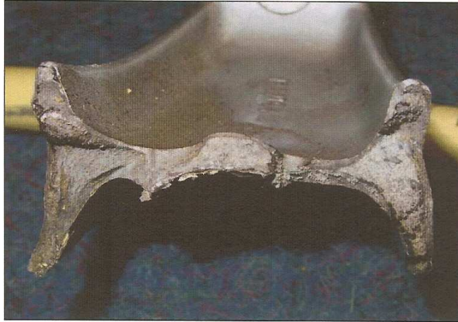
Figure 6. Fracture surface of the fractured blade horn (magnification: 1,2x).
