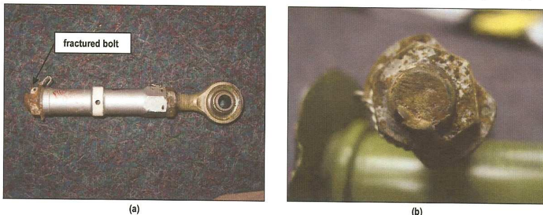
Figure 12. (a) The main rotor pitch change link in the as-supplied condition (magnification: 0,4x); and (b) an enlarged view of the fracture surface of the fractured pitch change link bolt (magnification: 1,5x).
