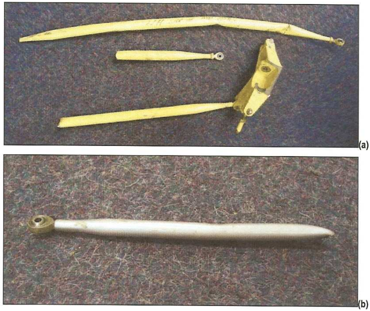
Figure 10. The fractured control rods supplied for examination: (a) magnification: 0,13x; and (b) magnification: 0,34x.
