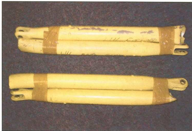
Figure 7. The main rotor gear box supports after removal from the salvaged wreck (top: left hand support; bottom: right hand support) (magnification: 0,16x).
