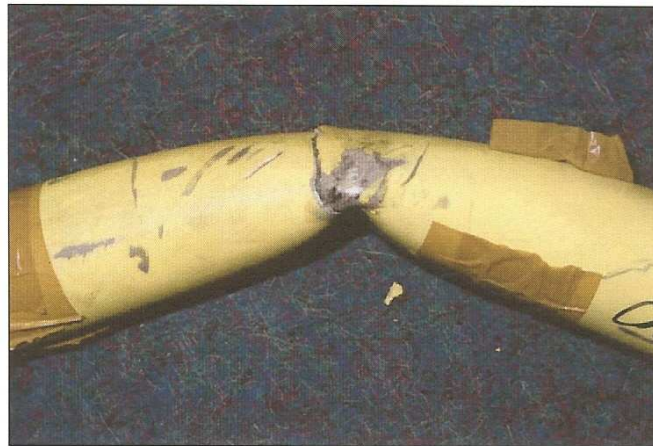
Figure 9. The two parts of the fractured left hand support lined up to illustrate that significant bending occurred prior to final failure (magnification: 0,47x).
