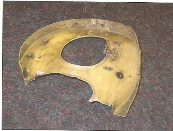
Figure 16. The damaged tail rotor gear box assembly in the as-supplied condition after removal from the wreck (magnification: approximately 0,2x).
