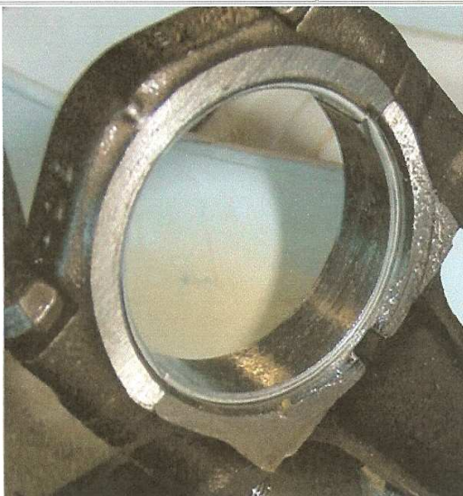
Photo 13: Intact con-rod from same engine (courtesy CAA)
