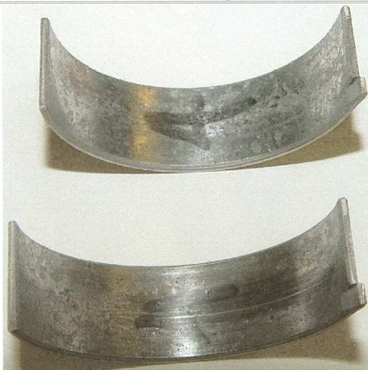
Photo 4: No 4 big-end bearing showing impregnation (digital)
