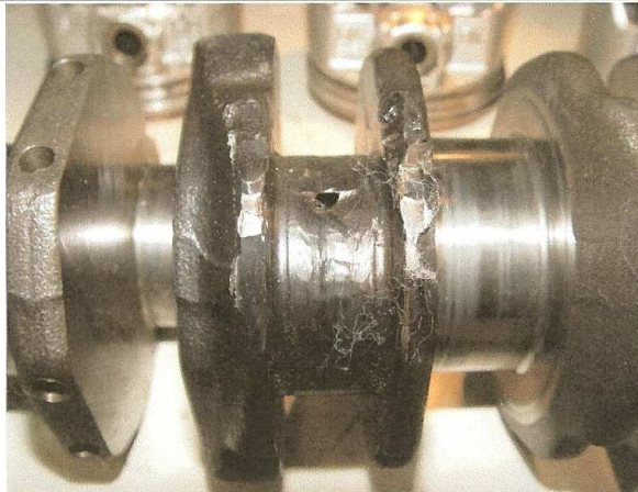
Photo 2: Crankshaft position of failure (digital)
