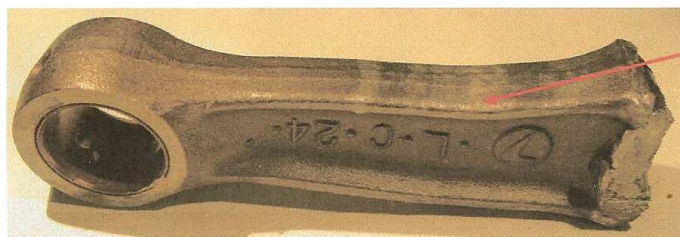
Photo 3: Con-rod showing bending and surface damages (digital)
