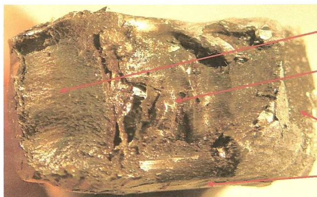
Photo 4: Con-rod fracture surface (digital)
