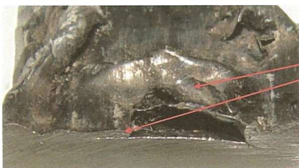
Photo 5: Failed con-rod end, sectioned to reveal layered bearing (digital)
