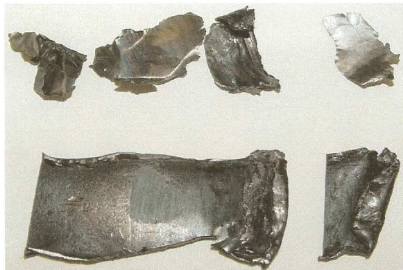
Photo 3: Remainder of big-end bearing (digital)
