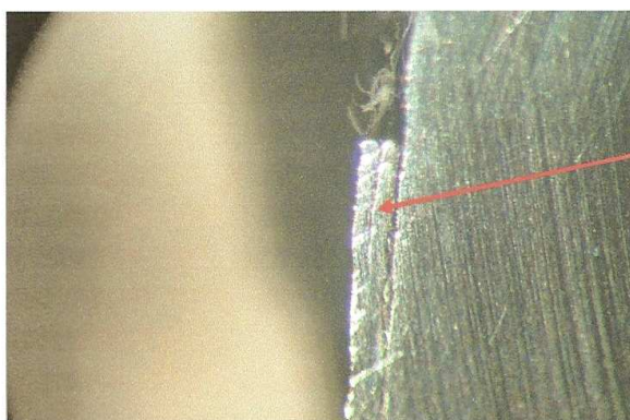
Photo 6: Layered bearing on failed con-rod big end (stereo)
