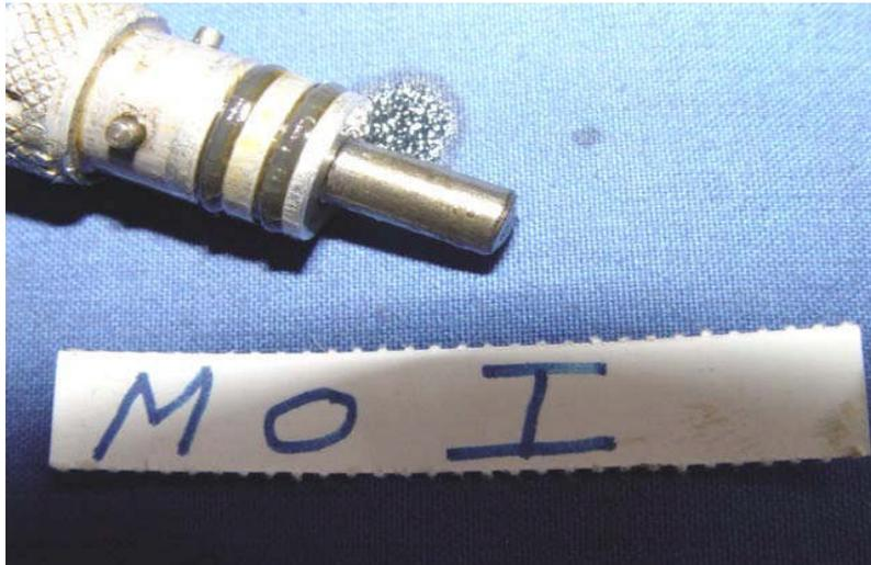
Figure 04: Transmission shaft and accessory gearbox (MO1) magnetic plug, free from magnetic particles
