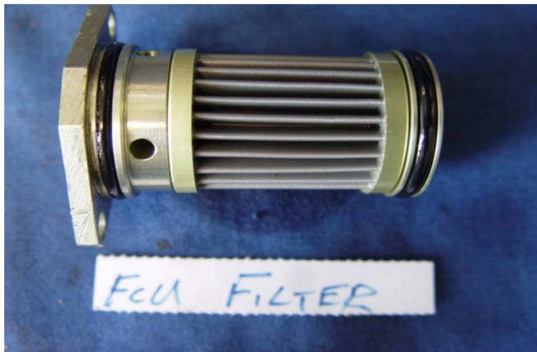
Figure 11: Fuel control unit filter element, contamination free.
