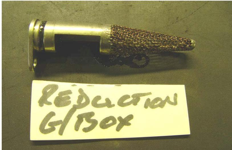
Figure 10: Reduction gearbox (MO5) oil return strainer, contamination free.
