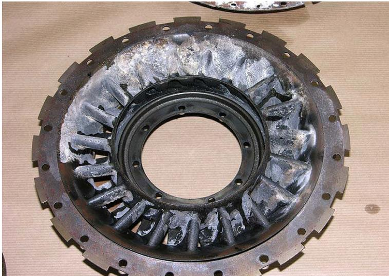
Figure 30: Gas generator turbine nozzle guide vane
