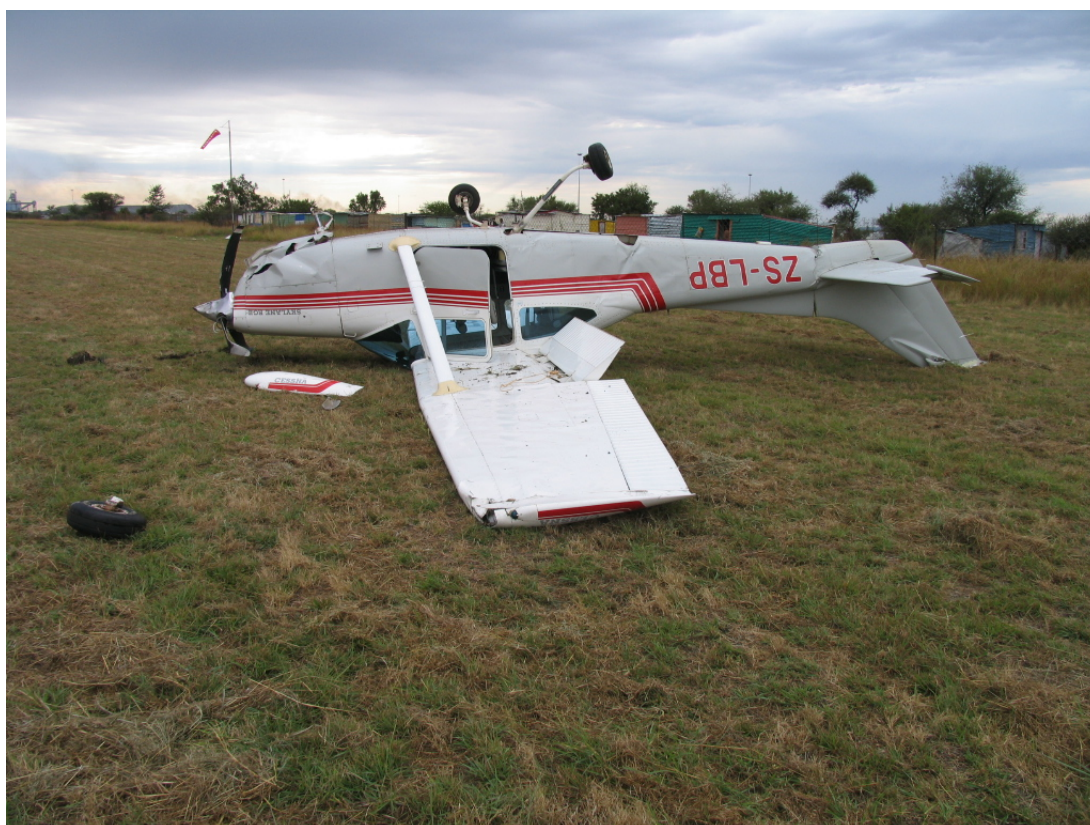
Figure 1. A view of the wreckage in an inverted attitude on the grass surface next to the runway.
