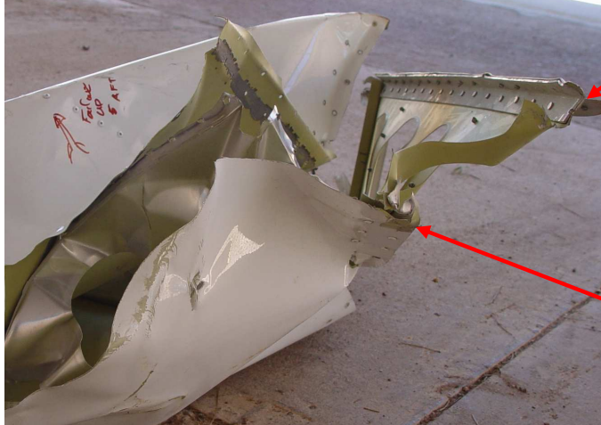
Photo 16: Right hand wing fractures at point C (digital)
