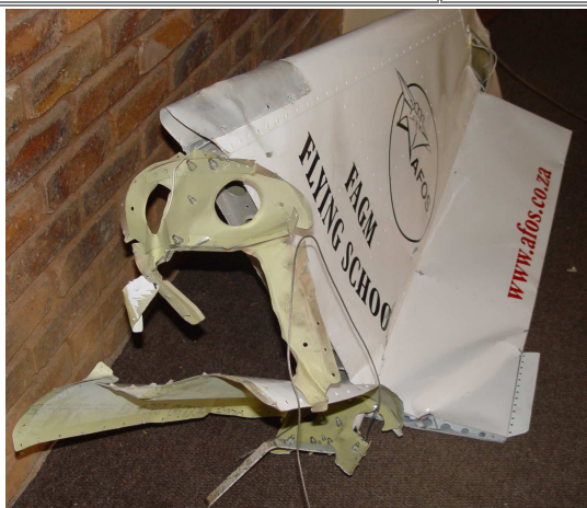
Photo 3: Rudder failure at point A (digital)
