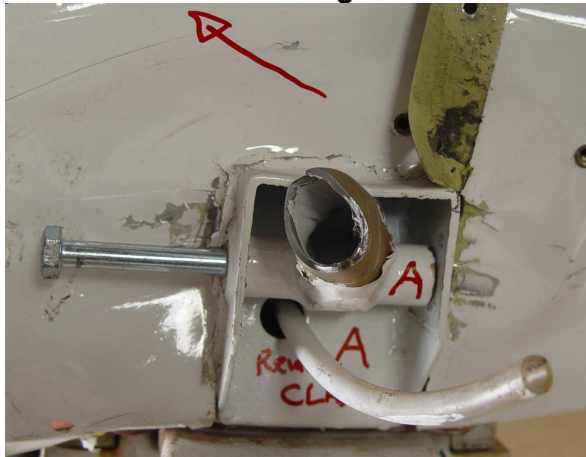
Photo 11: Left hand strut fuselage attachment at point D (digital)
