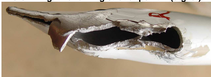
Photo 8: Right hand wing strut fracture surface (digital)
