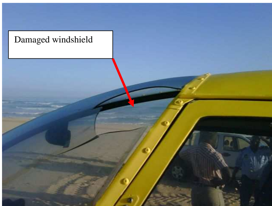
Figure 2: Damage to the left windshield
