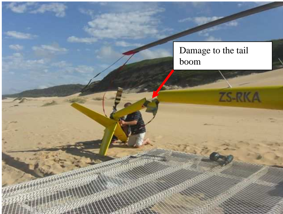
Figure 1: Damage to the tail boom
