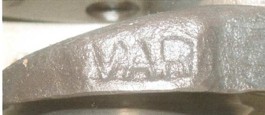
Photo 3: Crankshaft Vacuum Arc Re-melt stamp (digital)
