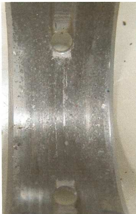
Photo 15: Main sleeve bearing surfaces showing metal impregnation (digital)
