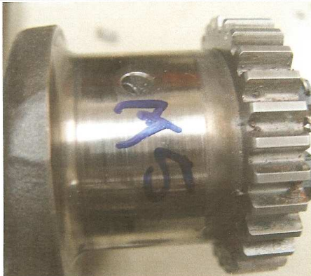
Photo 14: Condition of main bearing surfaces (digital)
