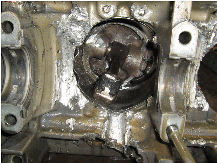
Figure 5: A view of the failed conrod (No. 5), with severe internal engine damage visible.
