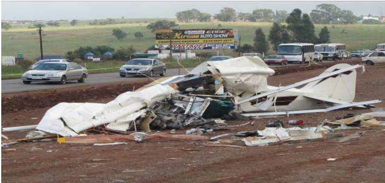
Figure 4: The main wreckage of the aircraft. The propeller blades indicated low rpm during the impact sequence
