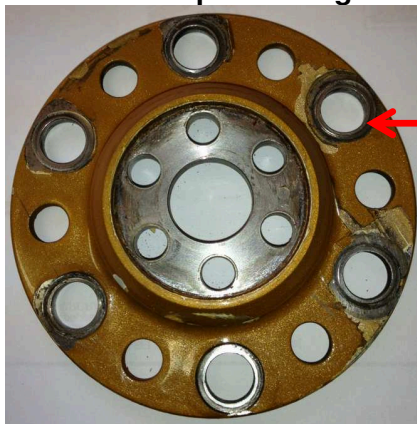
Photo 18: Propeller flange showing paint layer (courtesy Micro Aviation)
