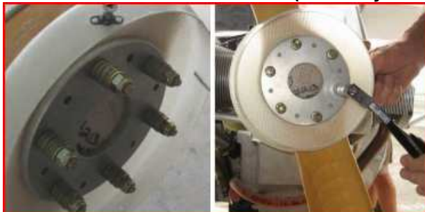
Photo 22: Fitment of Belleville washers and torque wrench application (courtesy Jabiru Constructors Manual)
