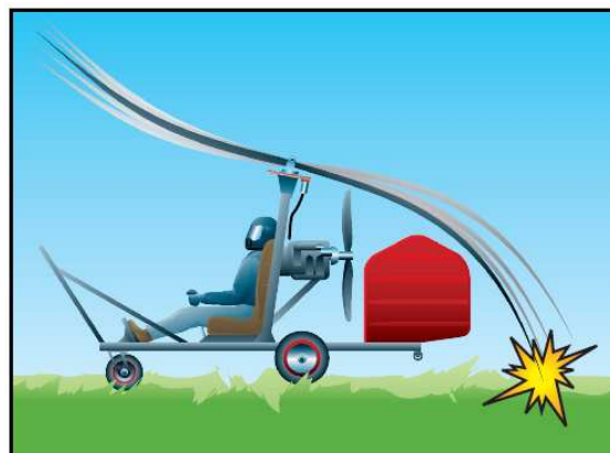
Figure 8: Taxiing too fast or gusting winds can cause blade flap in a slow-turning rotor. If not controlled, a rotor blade may strike the ground.
