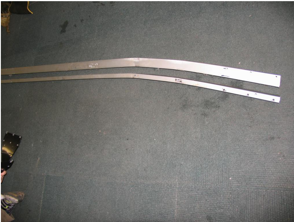
Figure 8. An indication of the bending the main mast suffered
