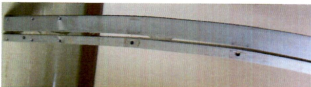
Photo 4: main rotor mast showing impact induced bending damages (digital)
