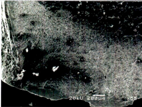
Photo 10: Fractograph, LF3 bolt hole (x55, SEM)
