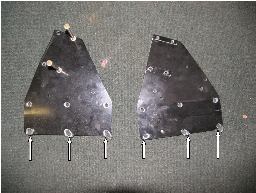
Figure 6. Deformation of the two attachment brackets after removal from the mast
