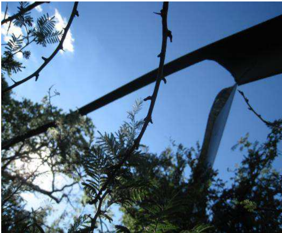
Figure 7: Destroyed main rotor.
