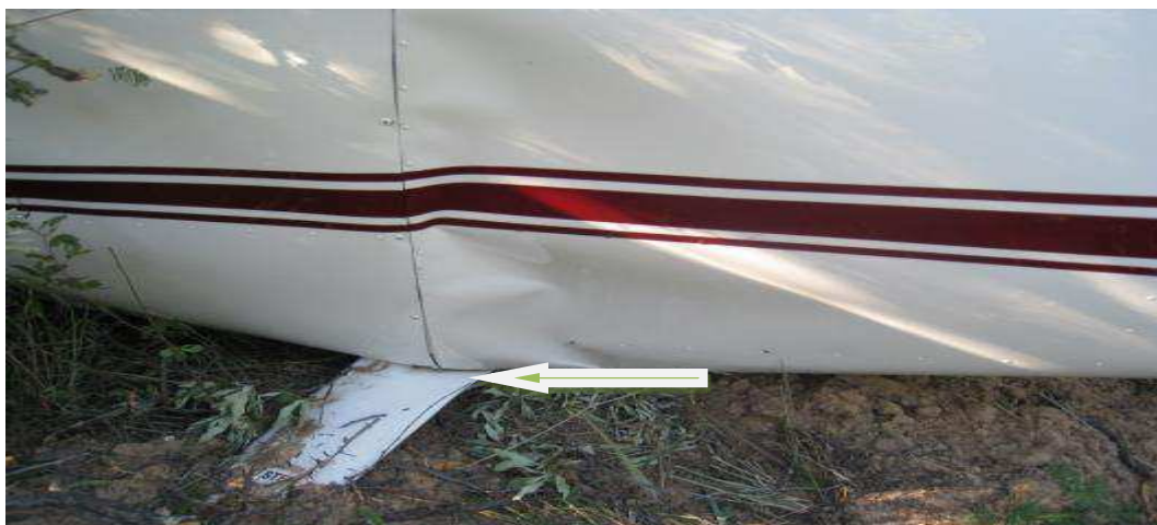
Figure 3: Evidence of damage to skids and airframe.
