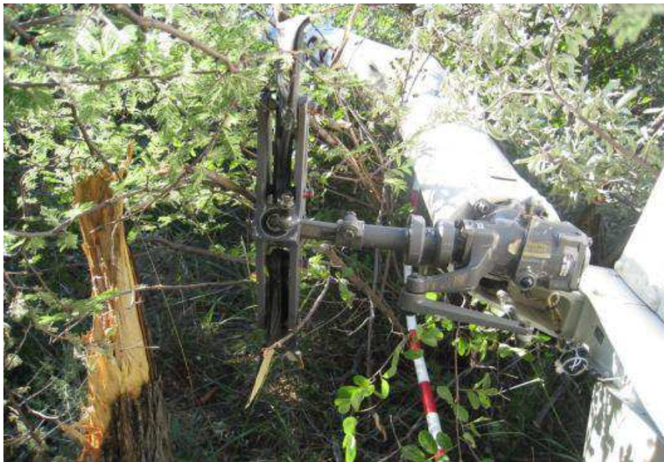
Figure 8: Severed tail boom.
