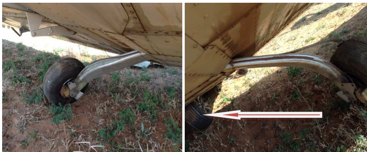
Figure 5/6: Damaged main landing gear with the nose wheel visible
