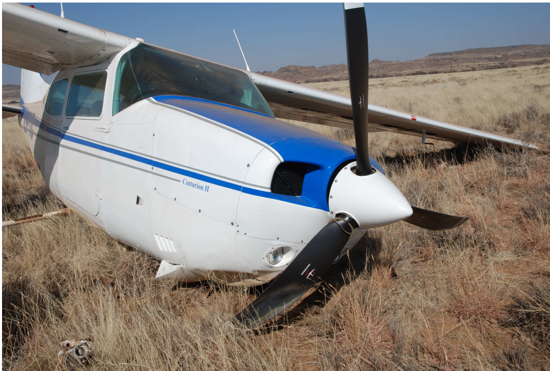
Figure 2: The damage to the propeller and dents on the lower fuselage can be seen here.
