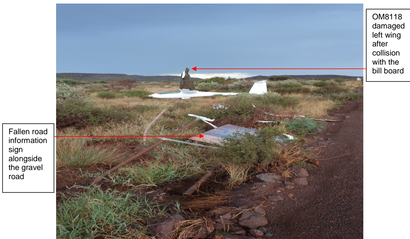
Figure 1: The final position of the glider after collision with the information sign
