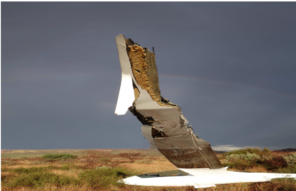
Figure 4: Damaged left hand side wing
