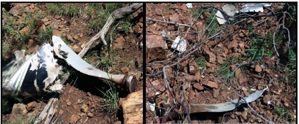
Figure 7: Shows damages on both propeller blades
