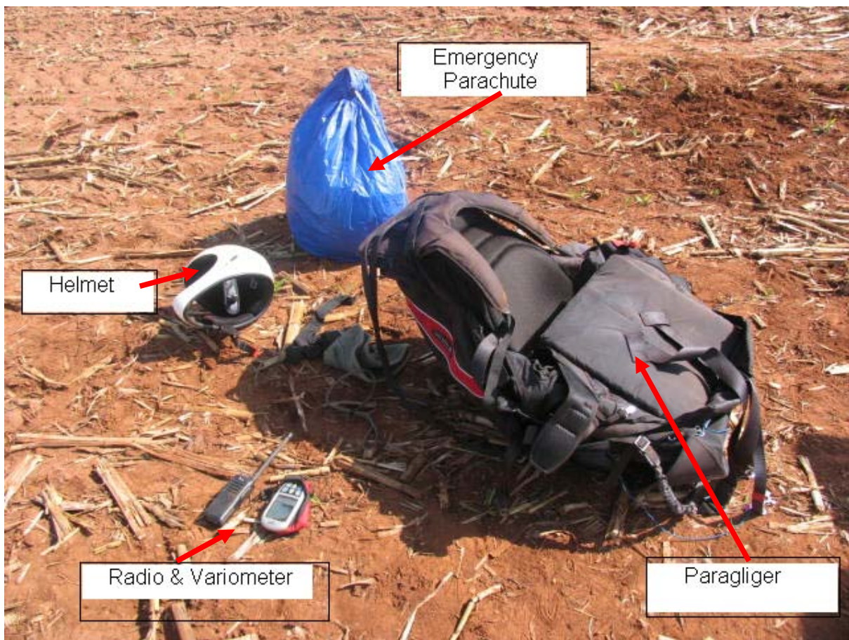
Figure 4. Paraglider equipment removed from the accident site.
