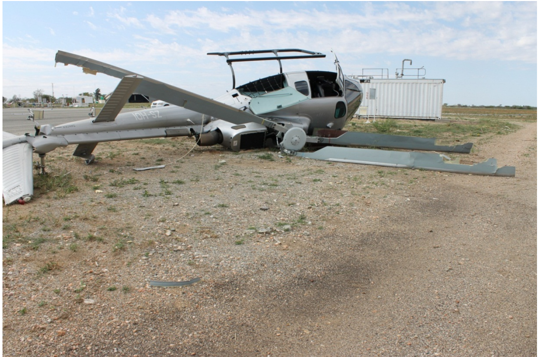
The damage to the main rotors suggests low rpm impact
