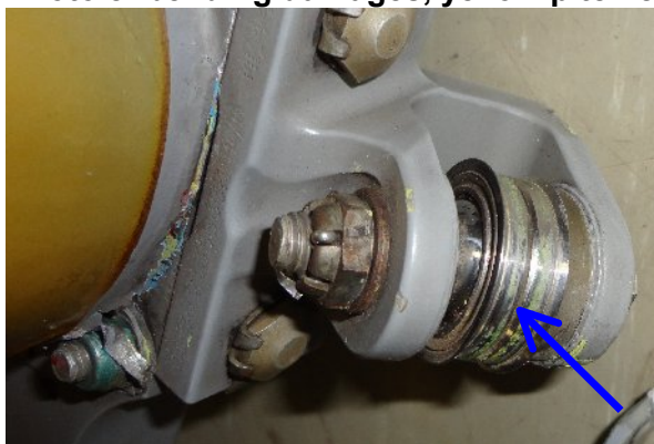
Photo 9: Big-end bearing at blade connector, yellow pitch control rod (digital)
