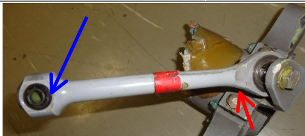
Photo 5: Impact marks, red pitch control rod (digital)
