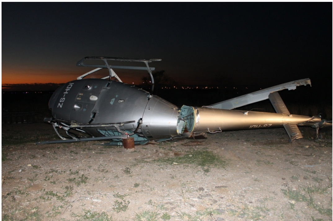
The cabin area was not extensively damaged by impact forces
