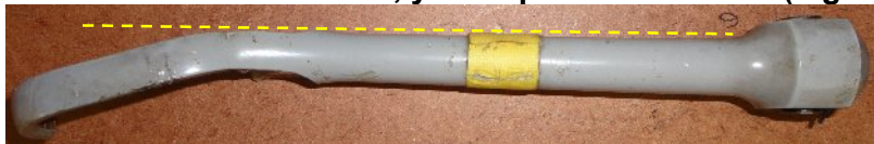
Photo 8: bending damages, yellow pitch control rod (digital)
