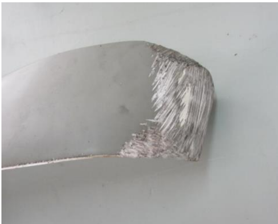
Figure 6: The propeller tip with scrape marks.
