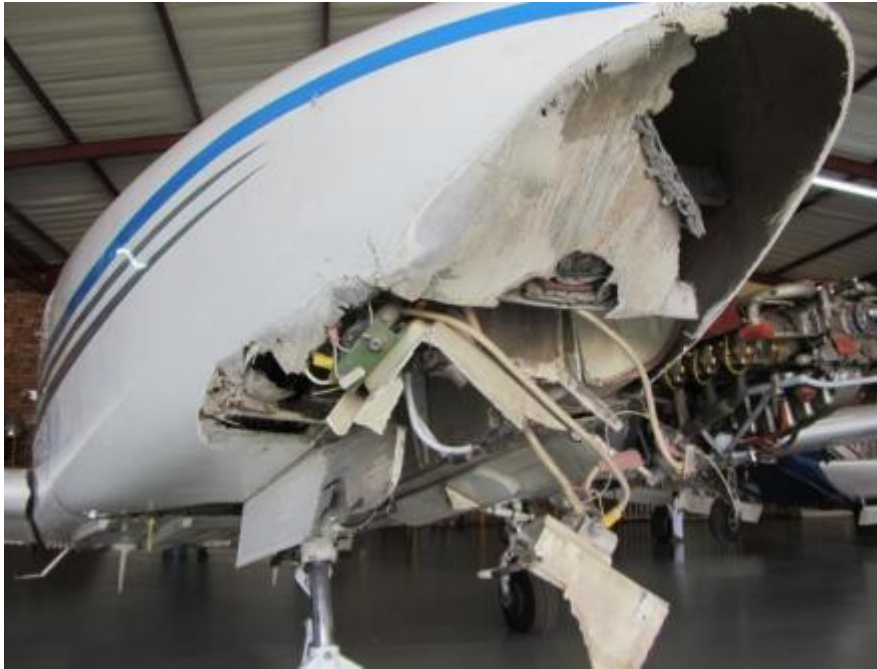
Figure 2: The damaged nose section.
