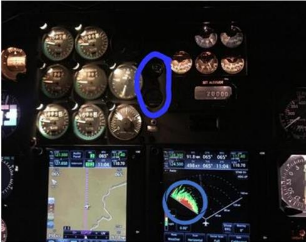
Figure 5: Emergency air unserviceable and radar paints left.
