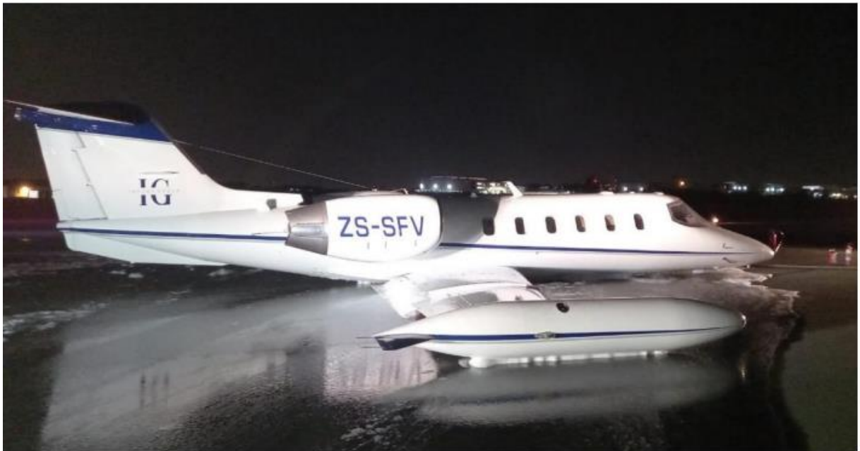
Figure 8: The ZS-SFV aircraft as it came to rest on its belly on the runway. (Source: AMO)
