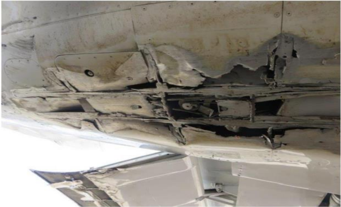
Figure 3: Damage to the underbelly and flaps.
