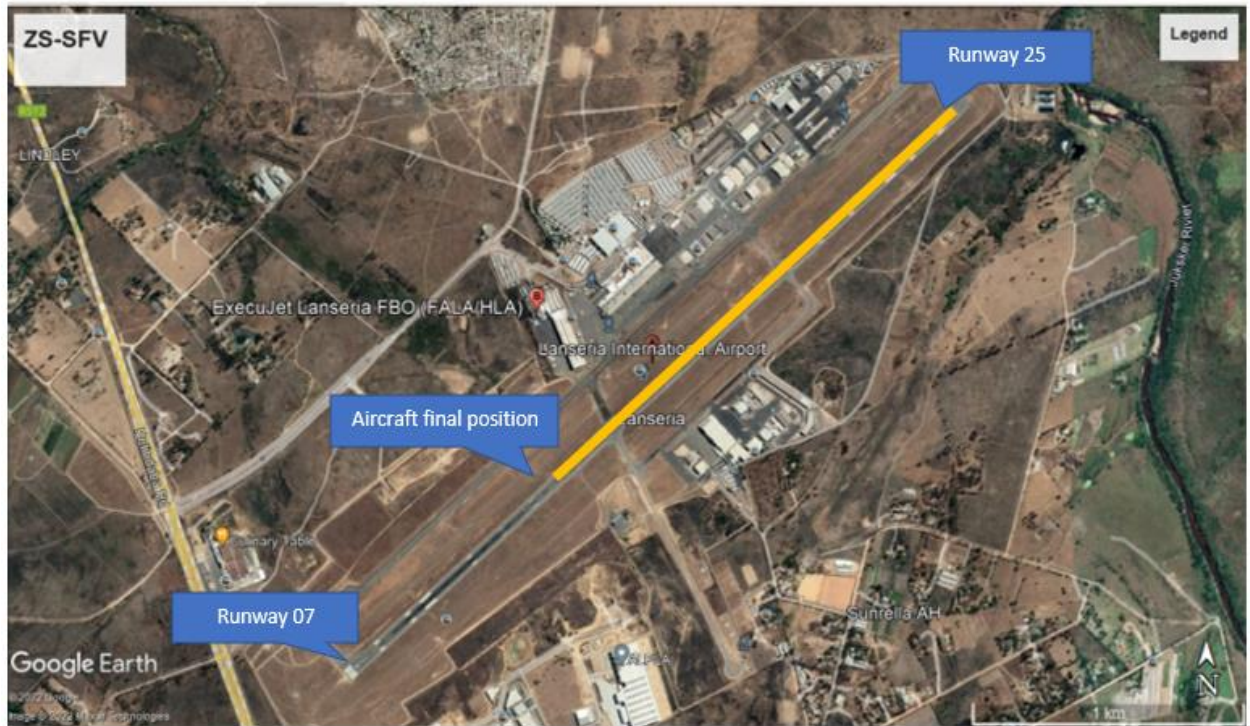
Figure 2: The approximate skidding distance of the aircraft during the accident. (Source: Google Earth)
