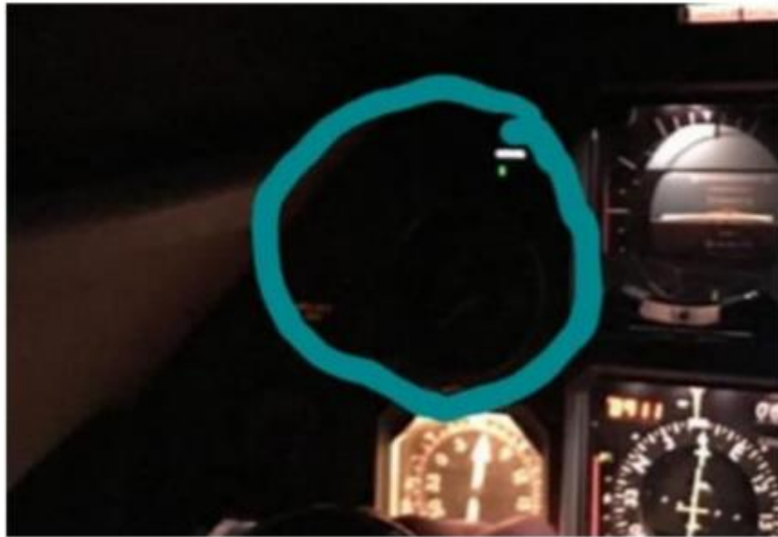
Figure 1: The air speed indicator backlight that was unserviceable.
