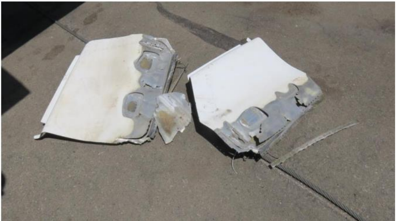
Figure 11: Damaged main landing gear doors.
