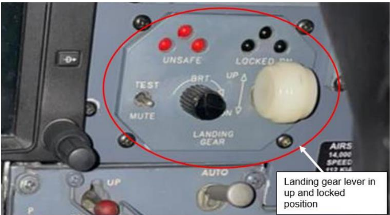
Figure 10: Landing gear lever in up and locked position. (Source: AMO)
