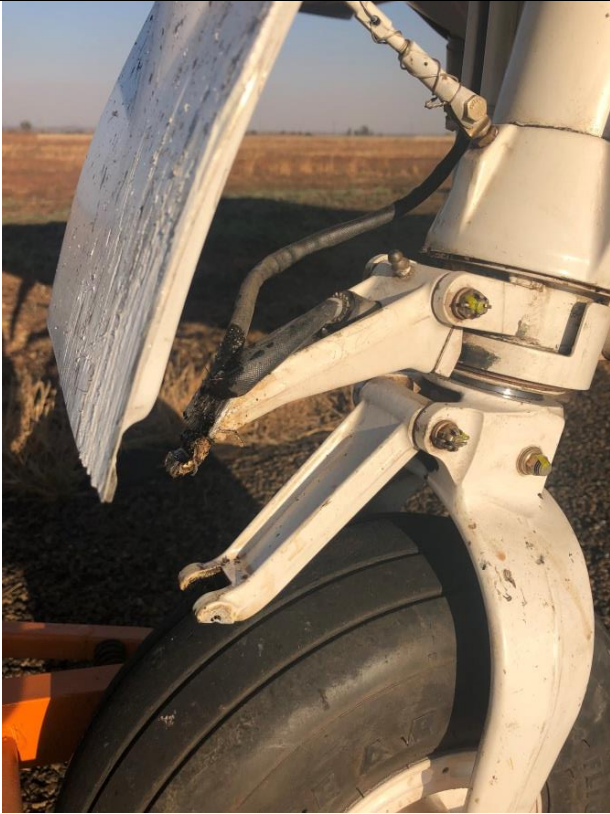
Figures 3 and 4: Damage to the nose gear (left) and skid marks on the runway surface (right).
