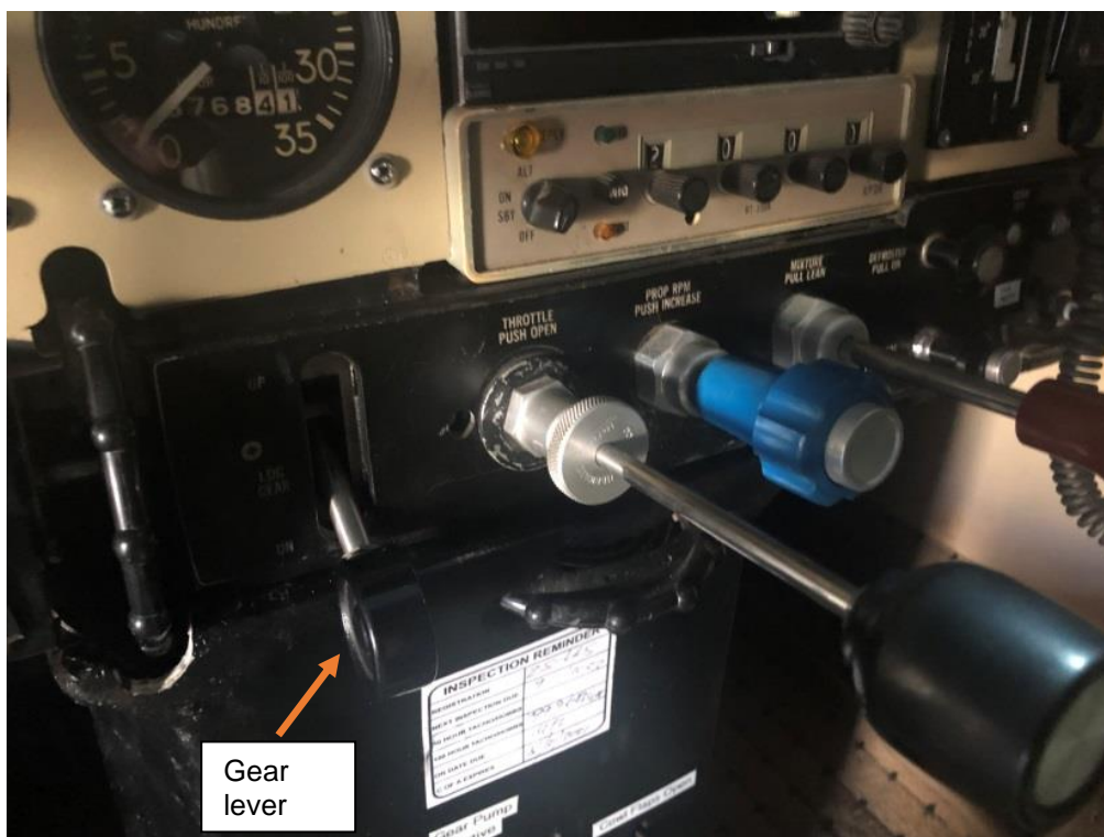
Figure 2: The gear lever when it is in the down and locked position. (Source: Pilot)
