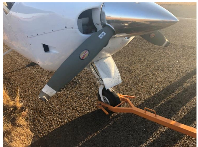
Figures 5 and 6: Damage on the exhaust (left) and propeller blade tips (right).
