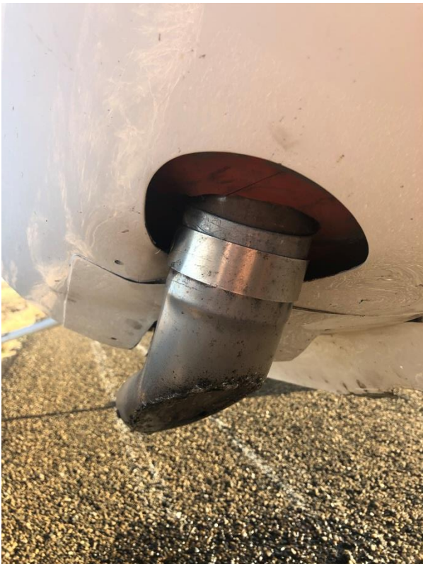
Figures 5 and 6: Damage on the exhaust (left) and propeller blade tips (right).
