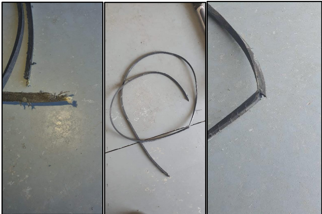
Figure 10: The V-belt condition at the accident site post-accident.
