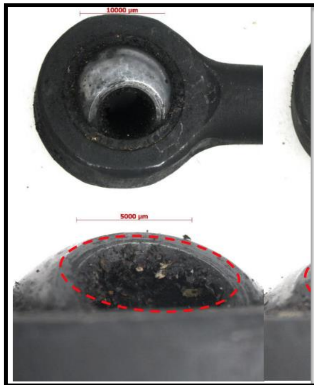
Figure 10: Ball-eye end and affected cable. (Source: University of Pretoria)
