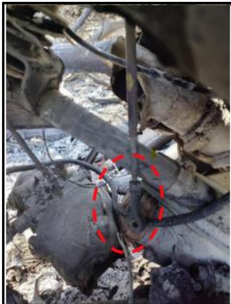
Figure 8: Throttle cable as found at the accident site. (Source: University of Pretoria)
