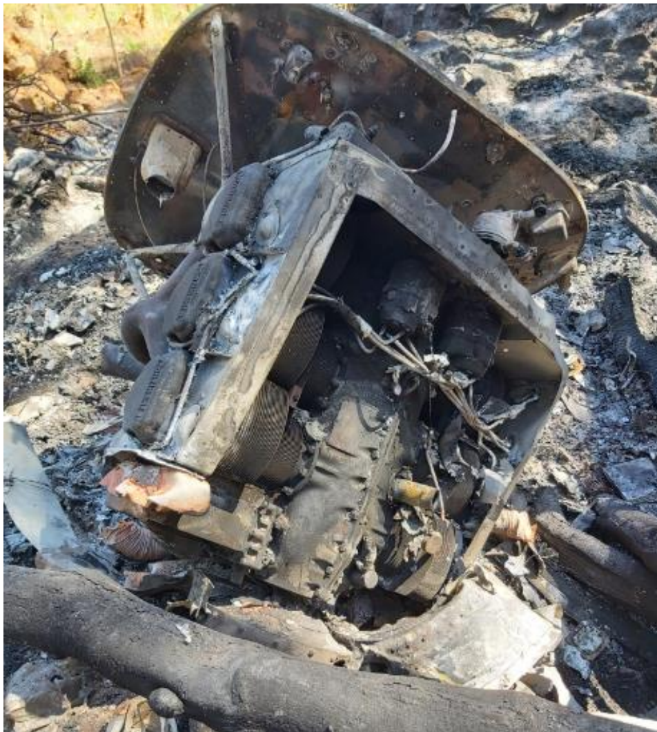
Figure 6: The engine and propeller blades post-accident. (Source: University of Pretoria)
