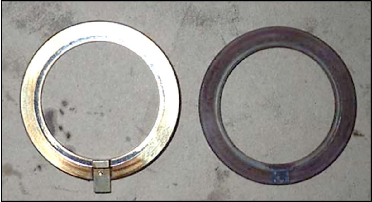
Figure 7: New thrust plate (left) and accident thrust plate (right) with a missing tab. (Source: Rolls Royce)
