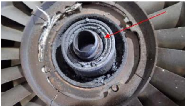
Figures 8 and 9: Thermal damage on the number 6 and 7 bearings. (Source: Rolls Royce)
