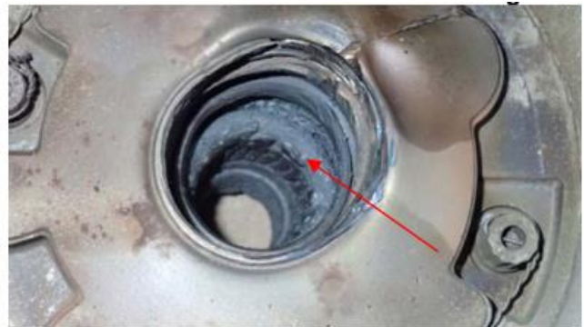
Figures 8 and 9: Thermal damage on the number 6 and 7 bearings. (Source: Rolls Royce)
