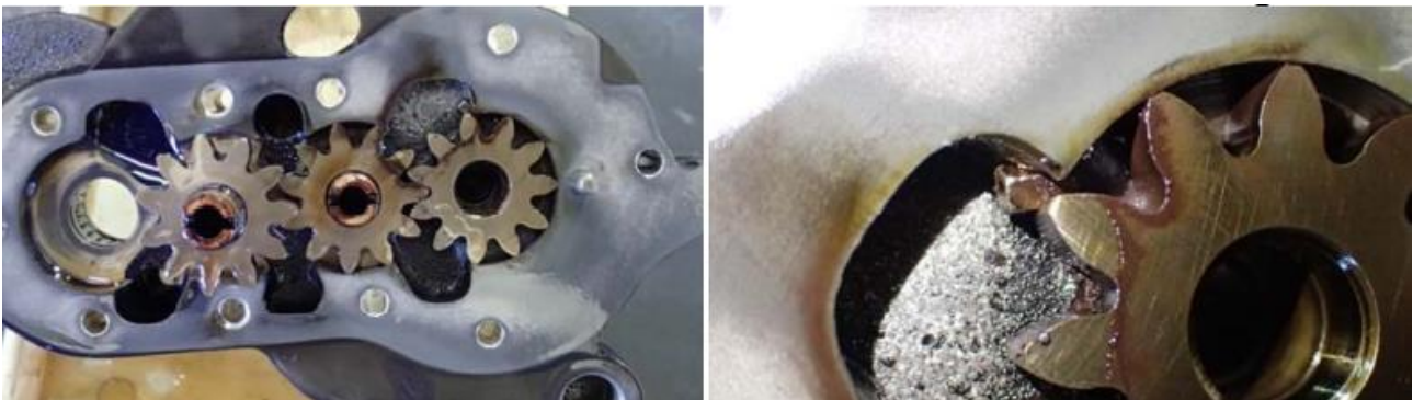
Figures 5 and 6: The oil pump scavenge gears with a tab lodged on the left gear. (Source: Rolls Royce)
