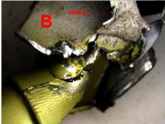
Photo 8: Sectioned fracture locations, inboard section (Stereo)
