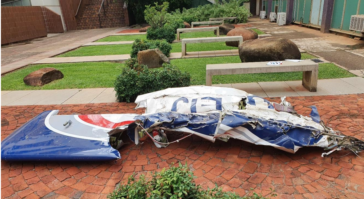
Figure 16: The left wing (both sections) positioned upside down.
