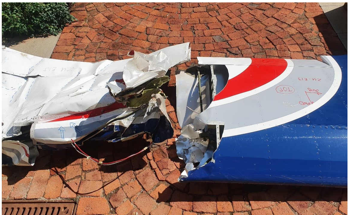
Figure 17: The area where the left wing failed is between ribs 8 and 9.
