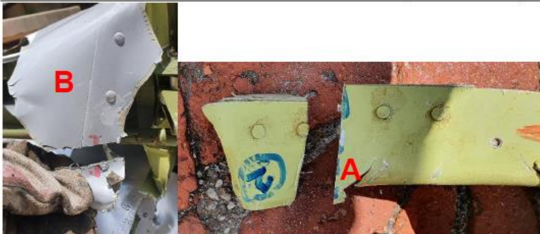
Photo 6: Sectioned fracture locations, outboard section (Stereo)
