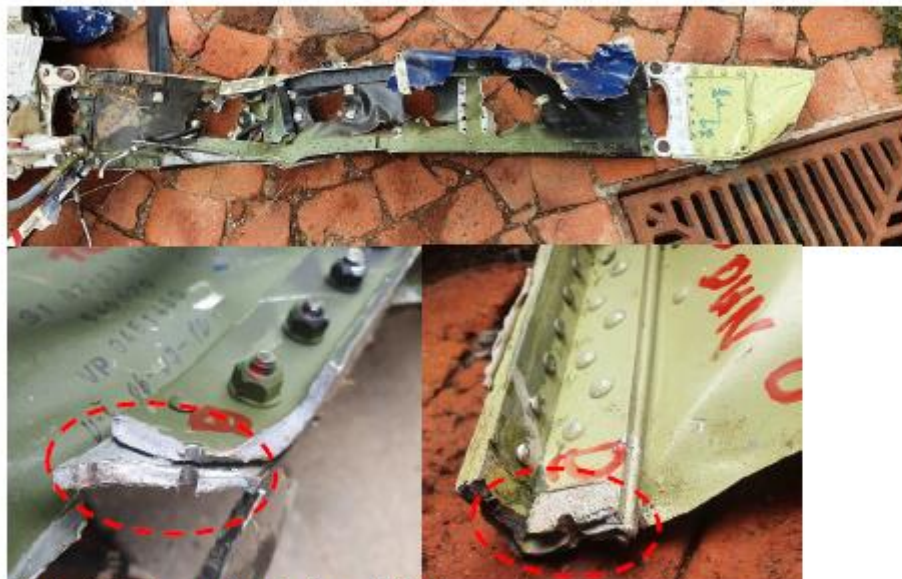
Photo 4: Centre section fractures (digital)
