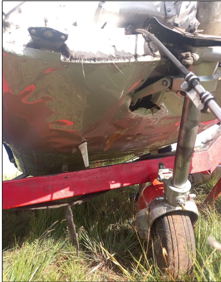
Figure 3: The nose landing gear strut that collapsed. (Source: Pilot)
