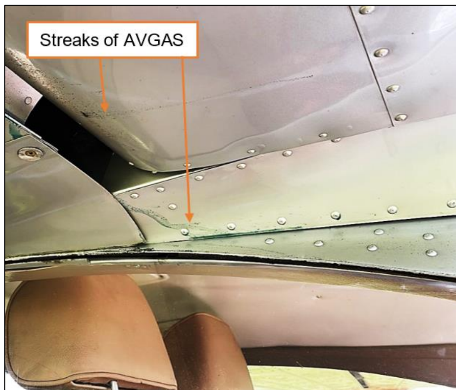
Figure 6: Streaks of AVGAS underneath the left fuel tank (left image) and along the roof of the cabin (right image). (Source: Pilot)
