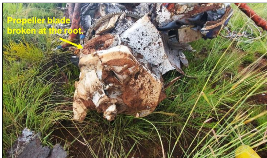
Figure 9: The propeller hub assembly.
