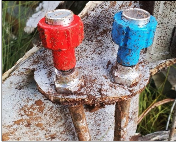
Figure 10: The throttle and mixture control/selecter levers.
