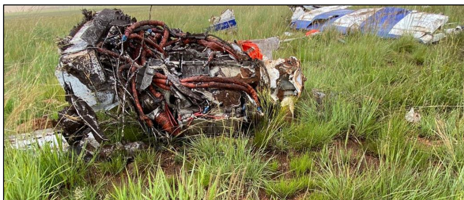
Figure 8: The condition of the engine and its proximity to the wreckage.
