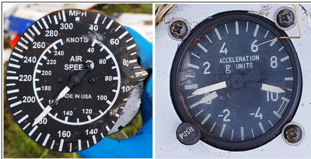
Figure 11: Airspeed indicator (left) and accelerometer (right).
