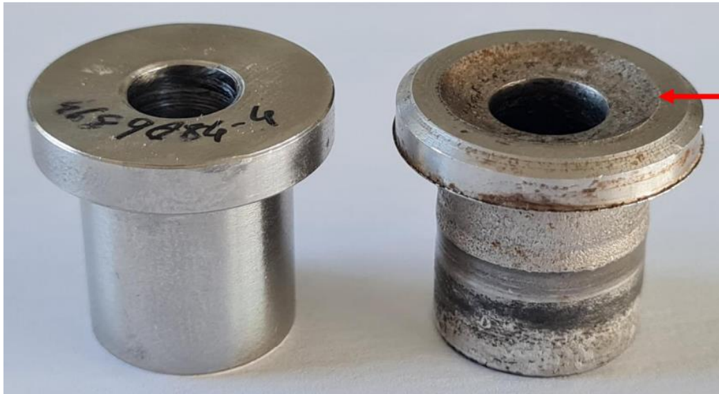
Figure 11: The pictures above were taken from the top and side angle. The new propeller bush is on the left and the bush from ZU-IKI is on the right. The wear on the bush from the AN5-42 bolt movement is clearly visible.
