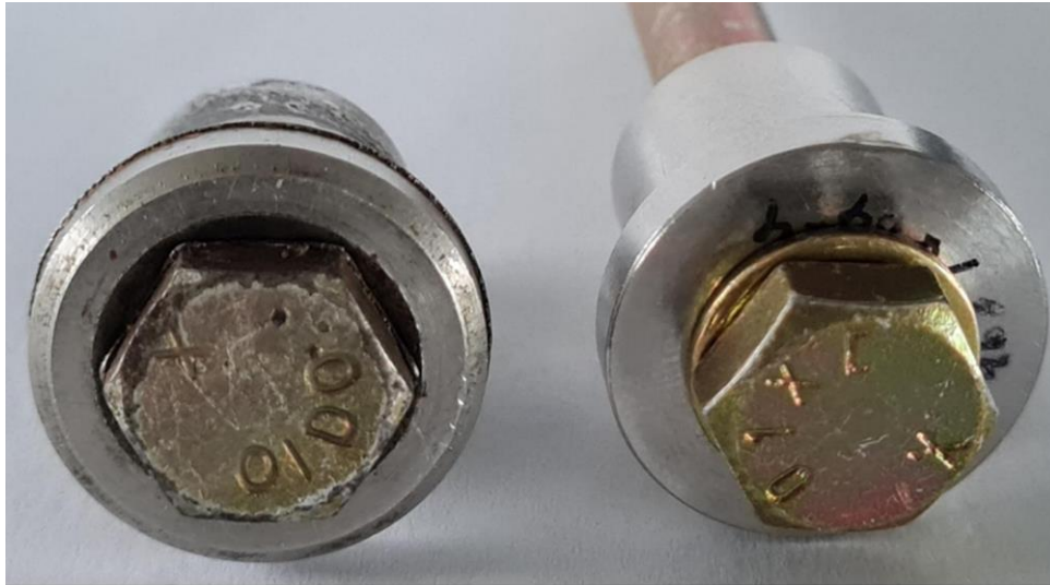
Figure 6: The AN5-42 bolt and the propeller bush from ZU-IKI (left), the new bolt and propeller bush (right).
