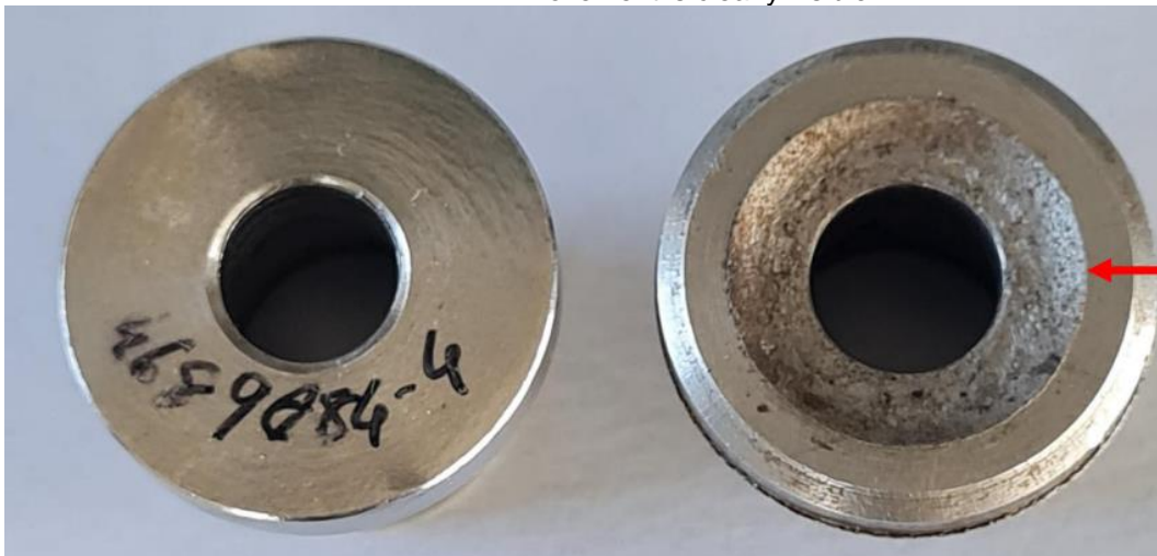
Figure 12: The two pictures show the propeller bush shaft taken from the side profile. The new propeller bush is on the left and the bush from ZU-IKI is on the right. The bush has been moving in the propeller hub as indicated by the striations on the bush shank.
