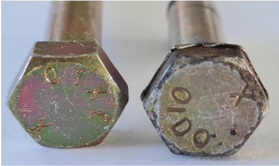
Figure 9: The heads of the AN5-42 bolt. The sheared bolt from ZU-IKI is on the right, showing the worn head.
