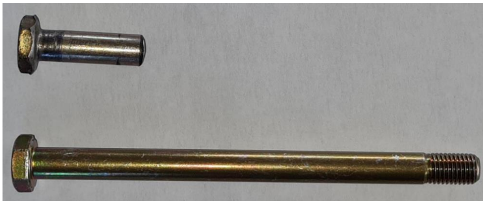
Figure 8: the AN5-42 bolt that was recovered (top) in comparison to the new bolt below (left).
