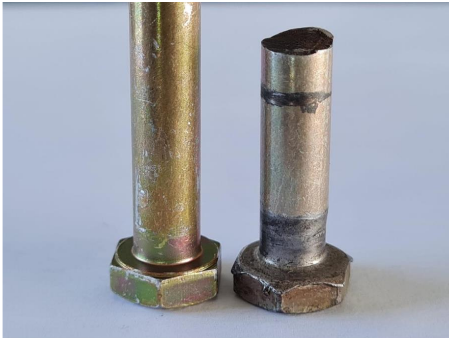
Figure 10: The AN5-42 bolt that had worn on the shank of the bolt as well as the head of the bolt which indicates movement.
