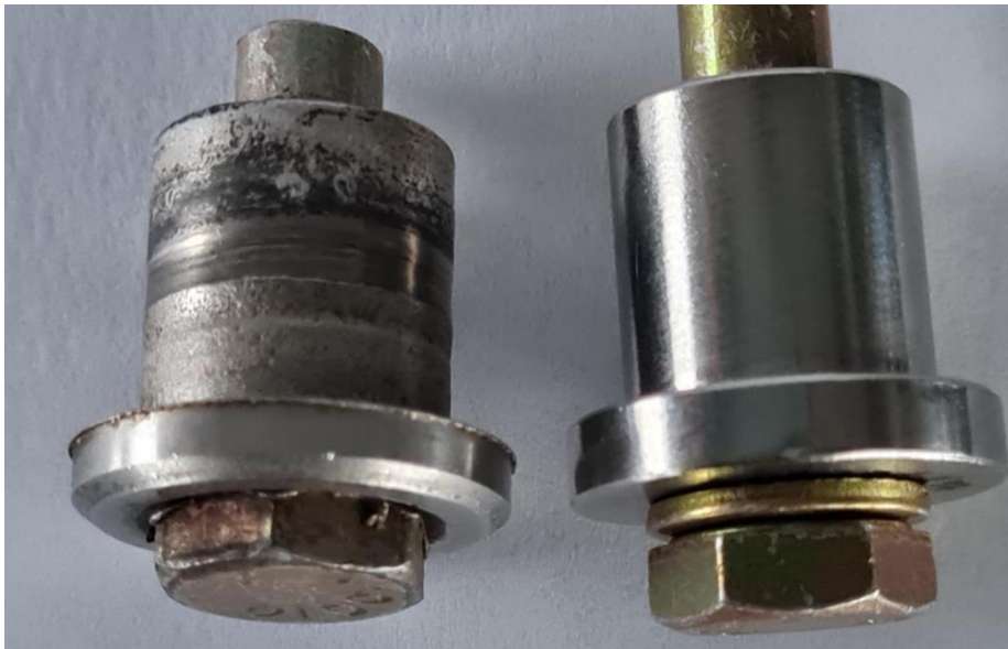
Figure 7: The head of the AN5-42 bolt from ZU-IKI (left) and the new item (right).
