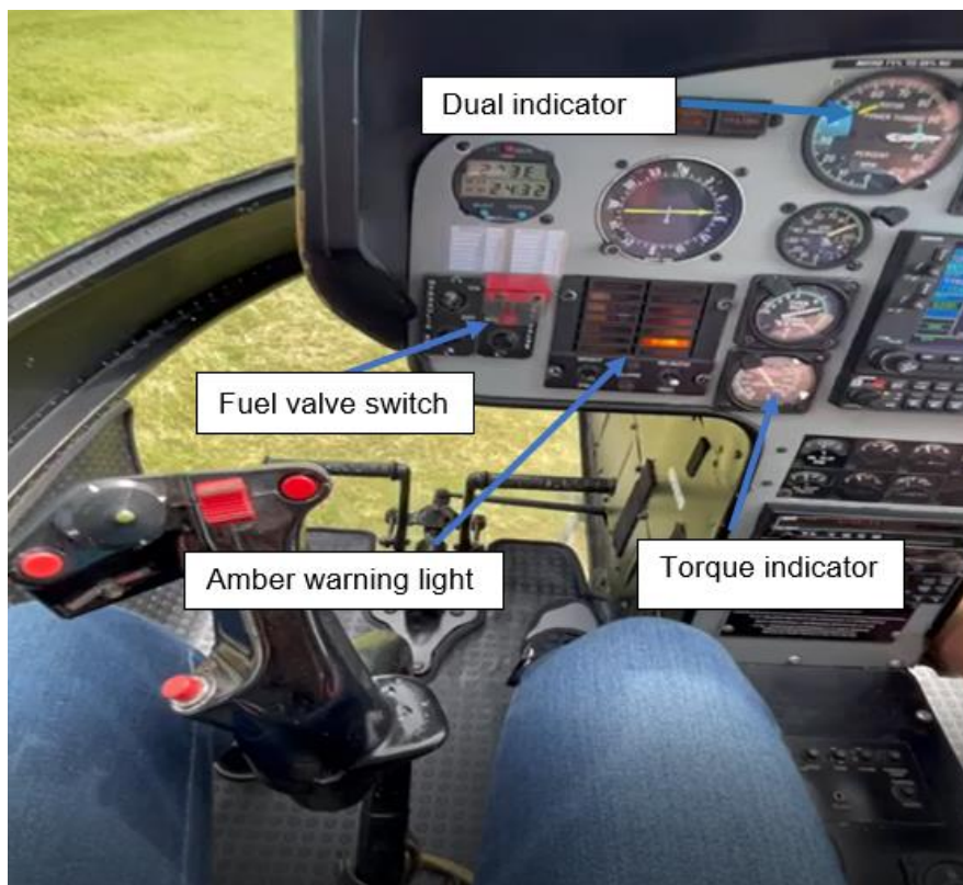
Figure 1: A video still showing arrows indicating positions of the fuel valve in the off position, torque indicator and dual gauge. (Source: Video footage from the passenger)
