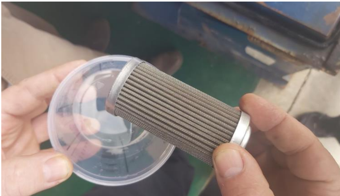
Figure 12: The condition of the fuel pump strainer after being removed from the pump assembly at the testing facility.
