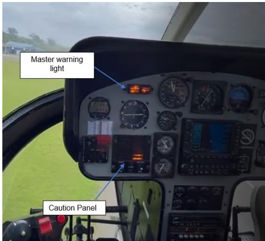
Figure 2: A video still showing master warning and caution as well as an additional caution message on the caution panel. (Source: Video footage from the passenger)
