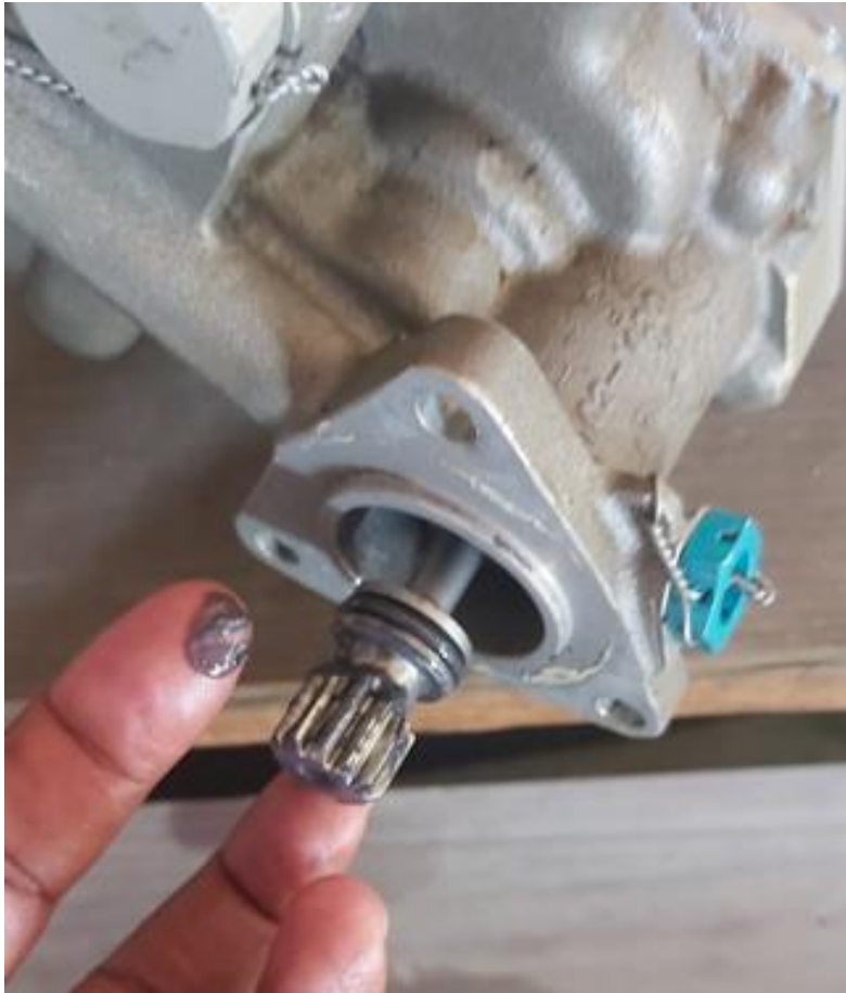
Figure 11: The shaft and the splines of the fuel pump.
