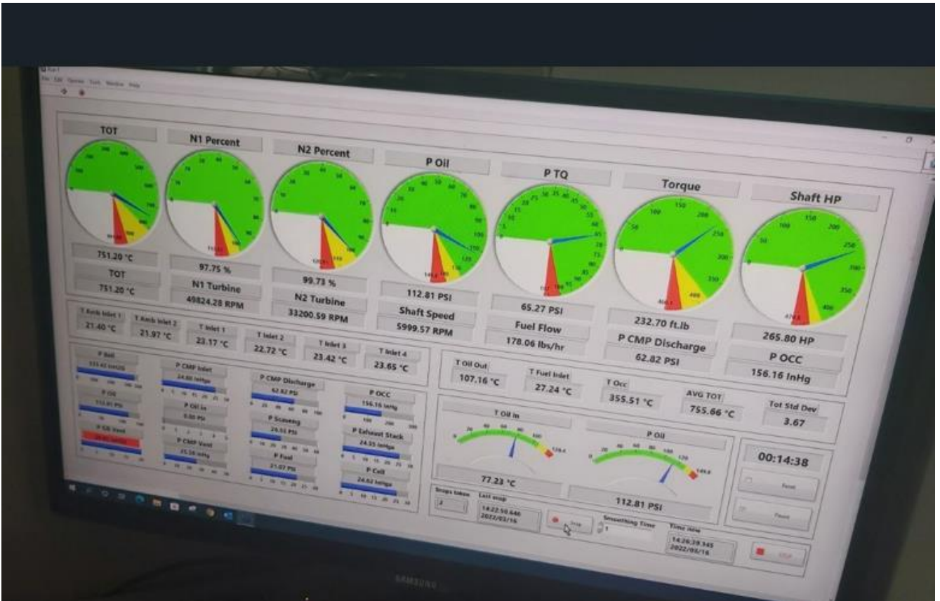
Figure 16: Screenshot of the engine parameters during bench testing.
