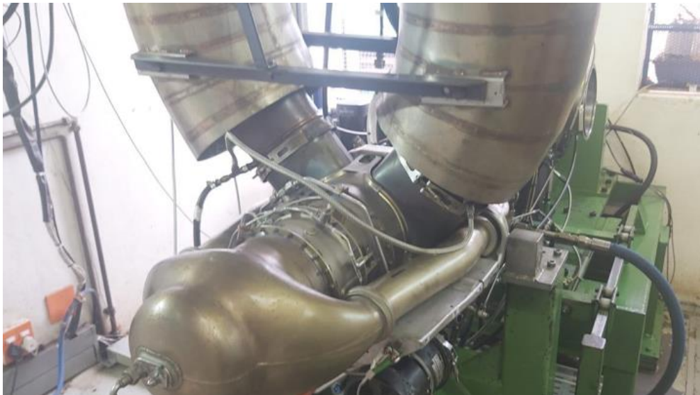
Figure 15: Accident engine fitted on a test bench.
