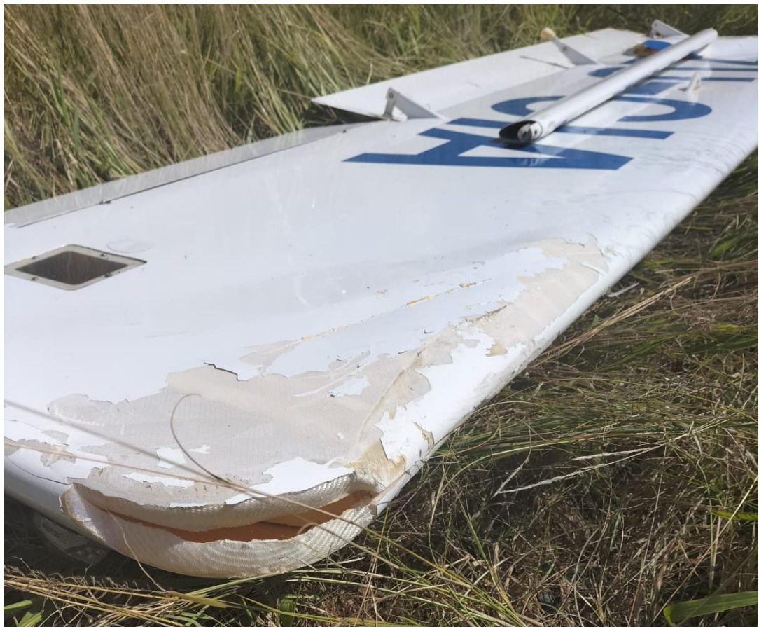
Figure 7: The damage to the left wing following impact with the road sign pole.
