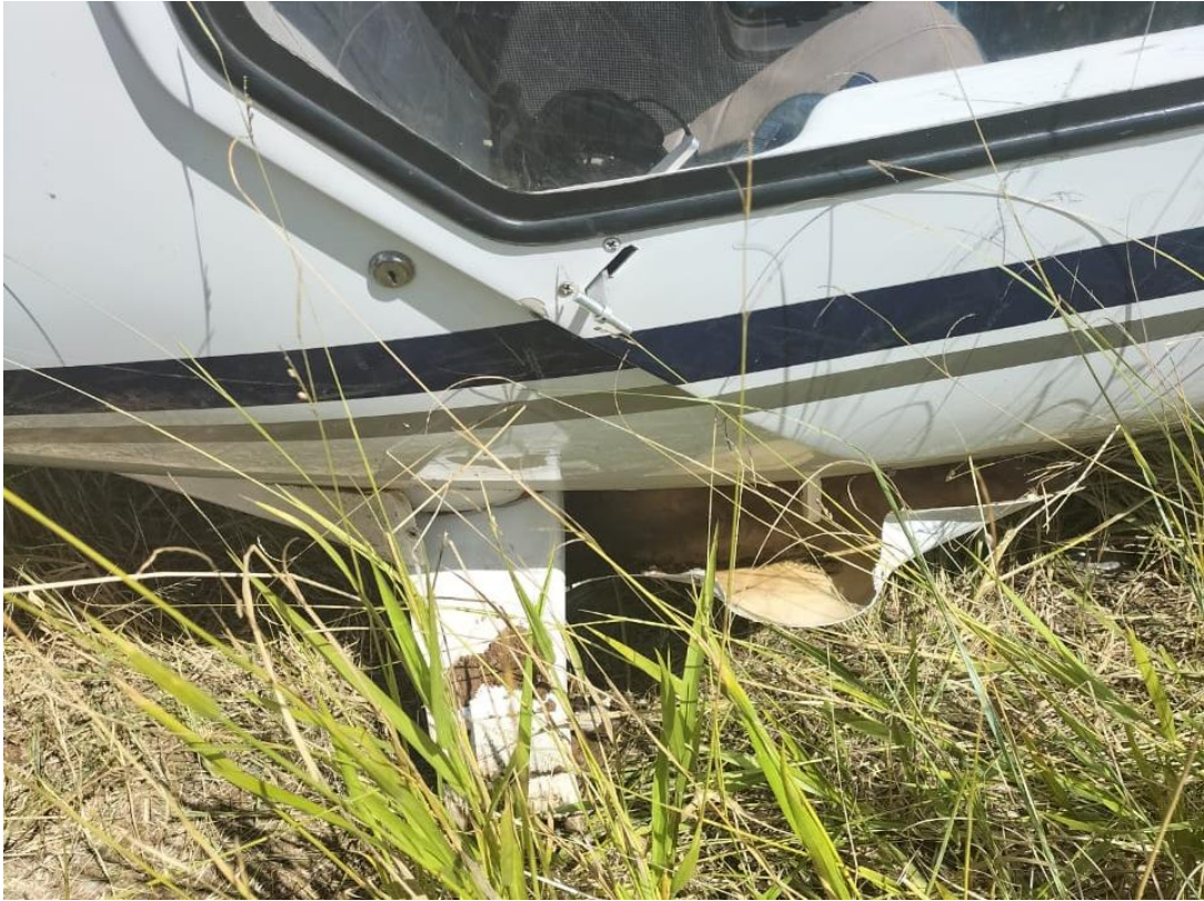
Figure 6: The right main gear strut broke off approximately midspan.
