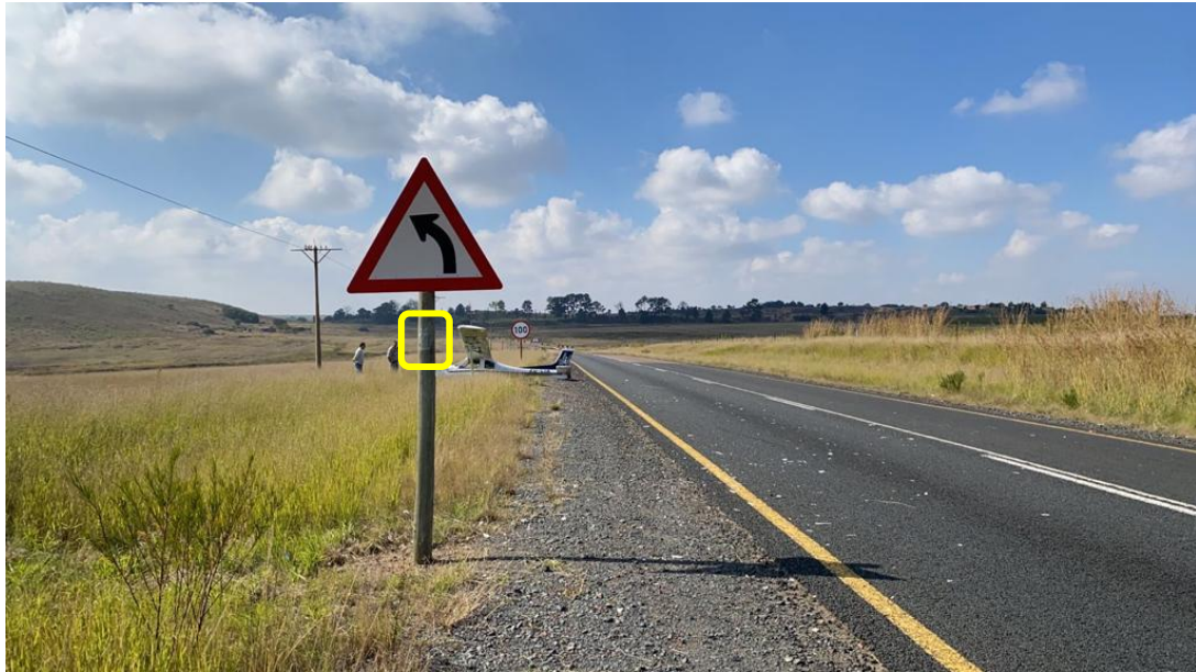
Figure 4: The road sign pole with which the aircraft's left wing collided, leaving a mark on it (see yellow block).
