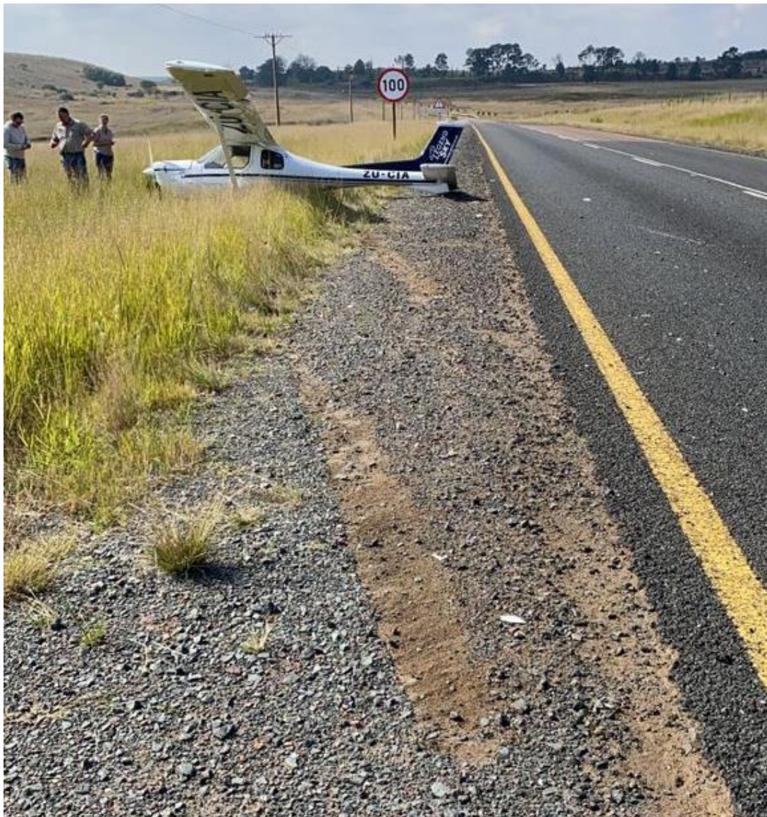
Figure 5: The tyre markings of the main wheels (both sides) as the aircraft veered off the roadway.
