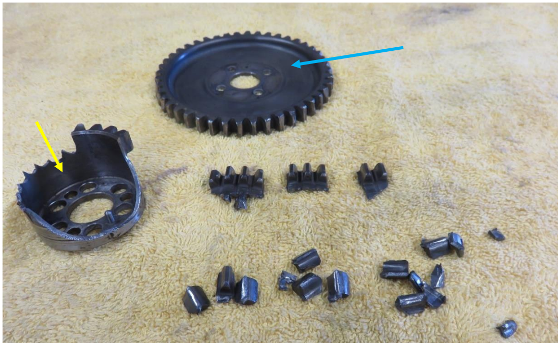
Figure 9: Fractured pieces from the crankshaft gear assembly and the flywheel (blue arrow).
