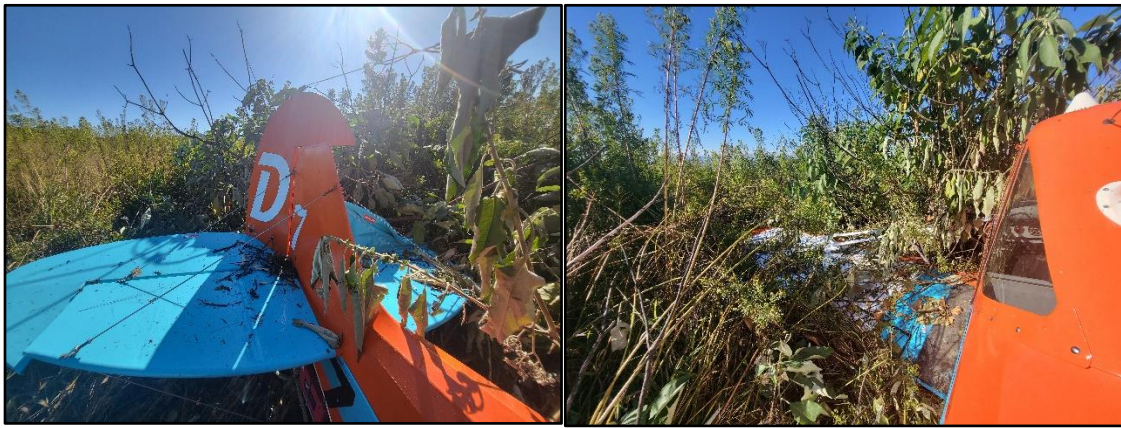
Figure 6 and 7: Damage to the left elevator (left); and left-side wing tucked in the bushes (right).
