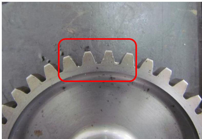
Figure 11: The crankshaft idler gear with wear on teeth. (Source: AMO)
