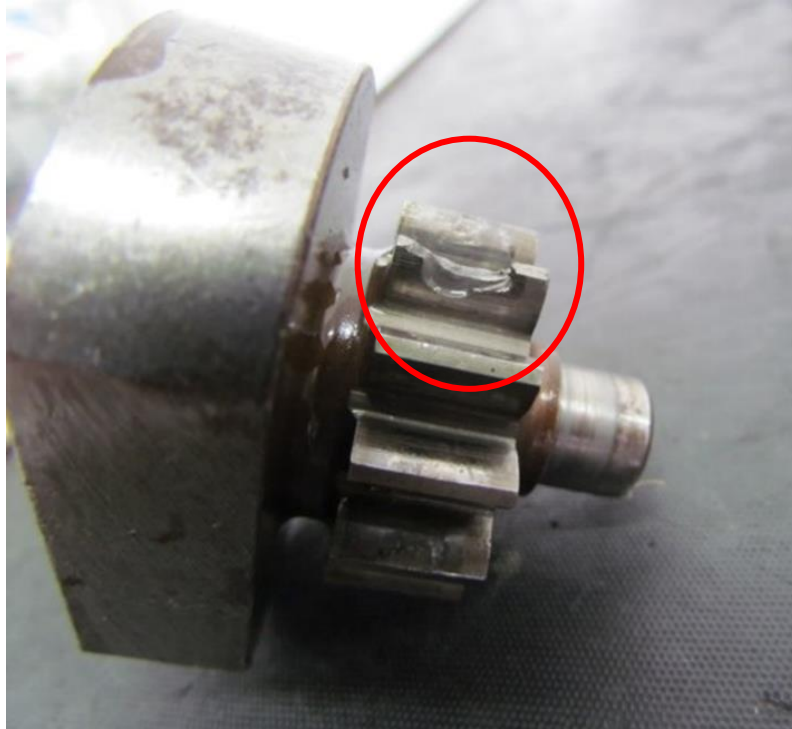
Figure 10: The left magneto drive gear indicating one of the broken teeth. (Source: AMO)
