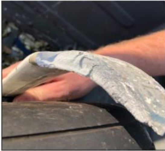
Figures 4 and 5: The clean breaks with no signs of pre-existing cracks. (Source: Operator)
