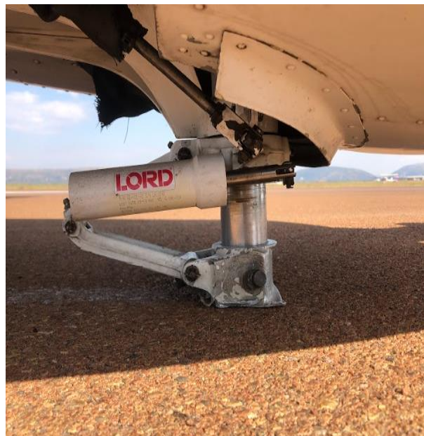
Figure 3 The break occurred above the nose wheel fork.
