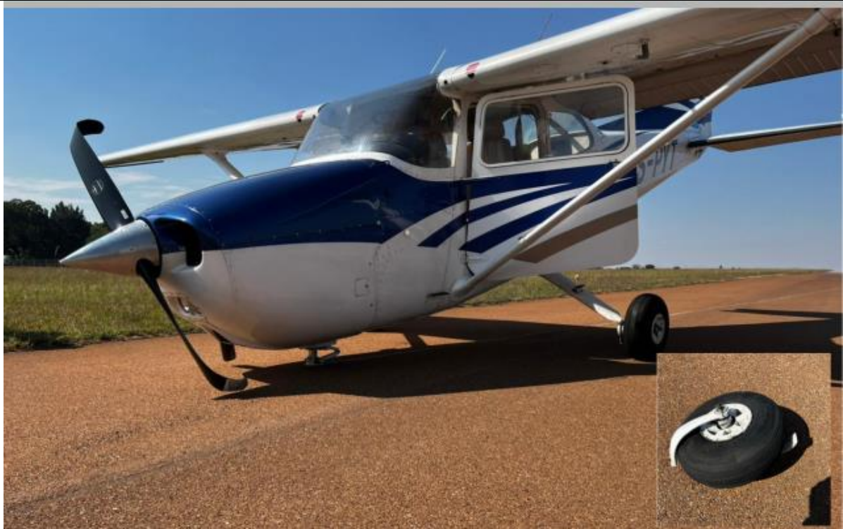
Figure 1: The aircraft on the runway with the broken nose wheel. (Source: Operator)
