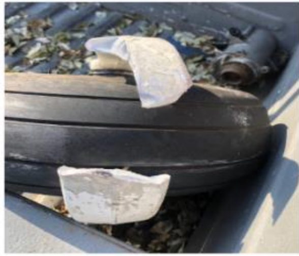
Figures 4 and 5: The clean breaks with no signs of pre-existing cracks. (Source: Operator)
