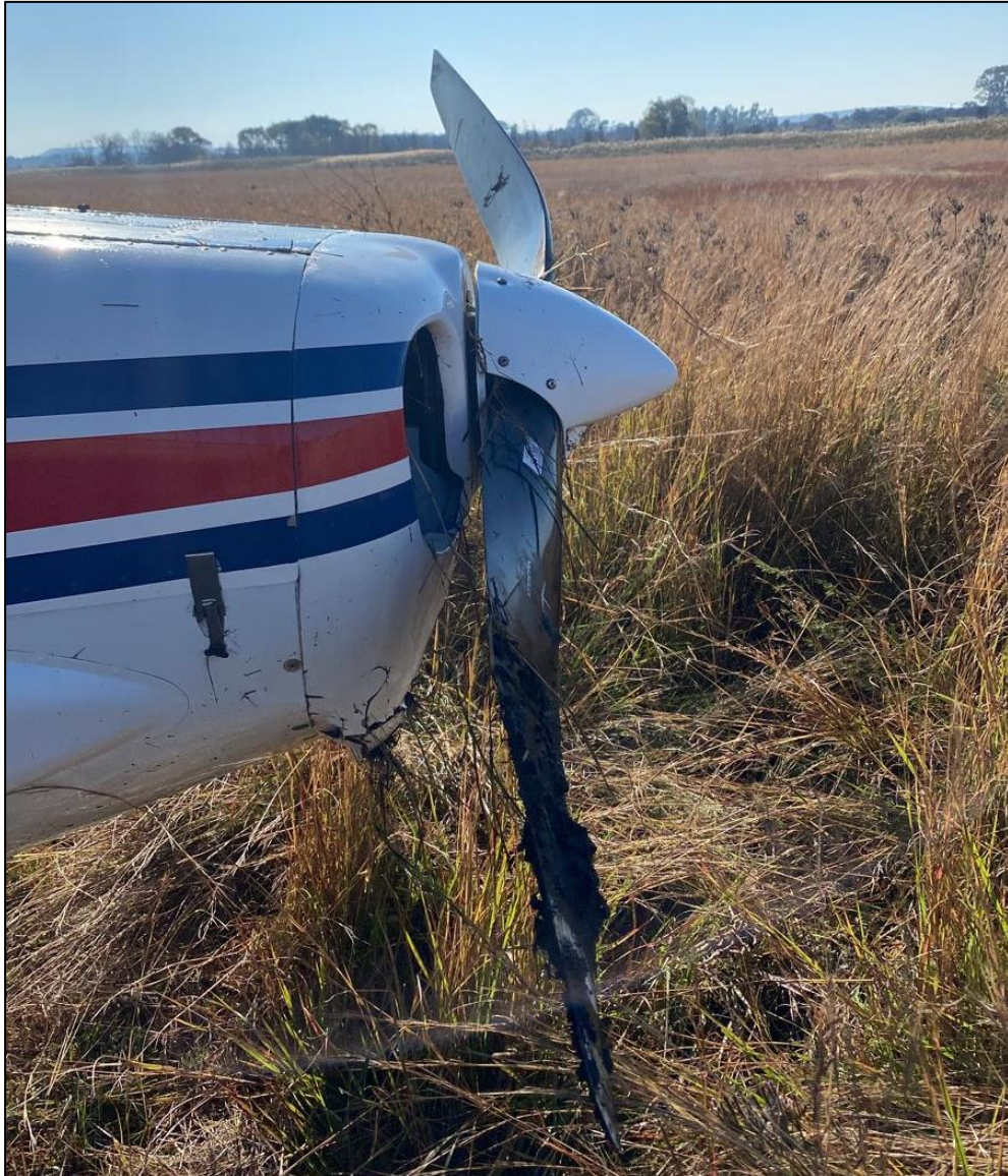
Figure 5: The propeller blades after the accident. (Source: AMO)
