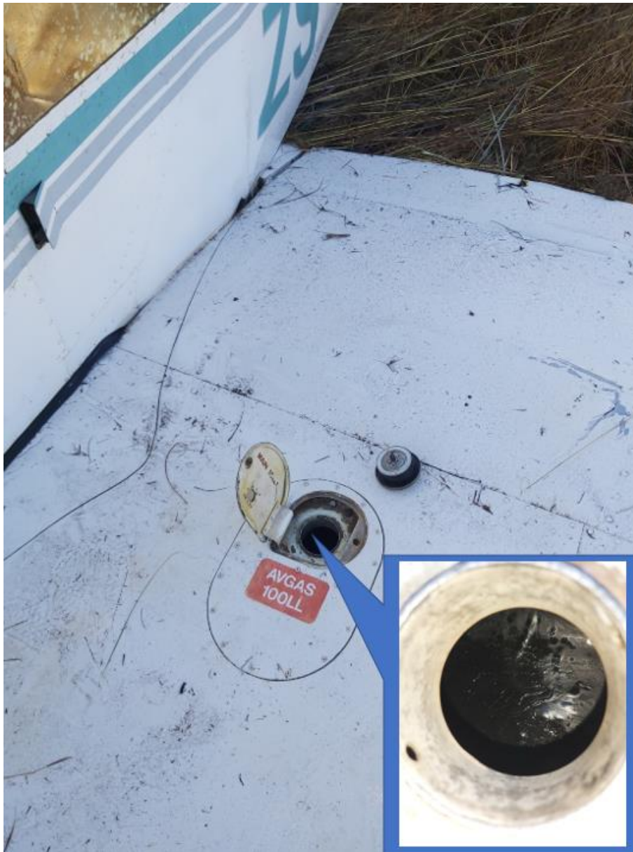
Figure 9: The left main fuel tank with no fuel.
