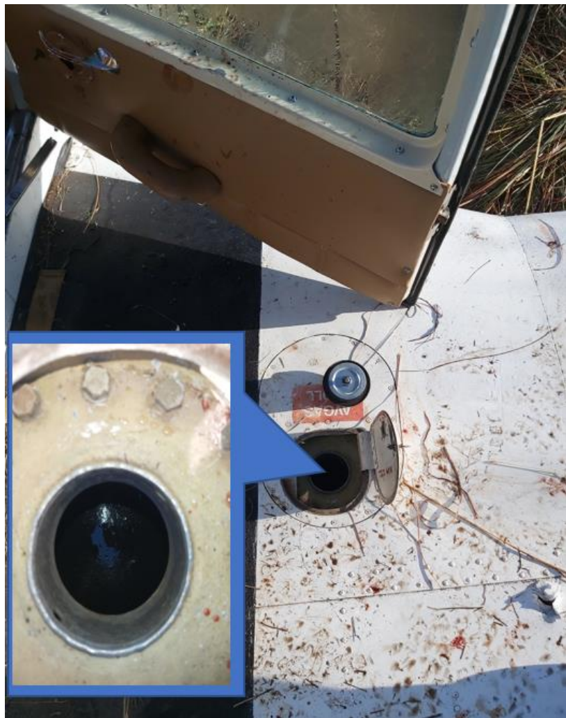
Figure 8: The right-side main fuel tank with no fuel.
