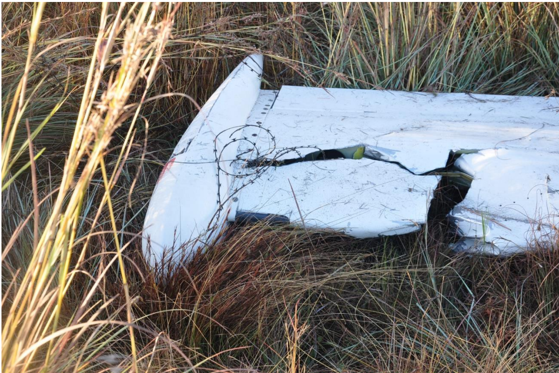
Figure 6: The right wing that impacted the fence post.
