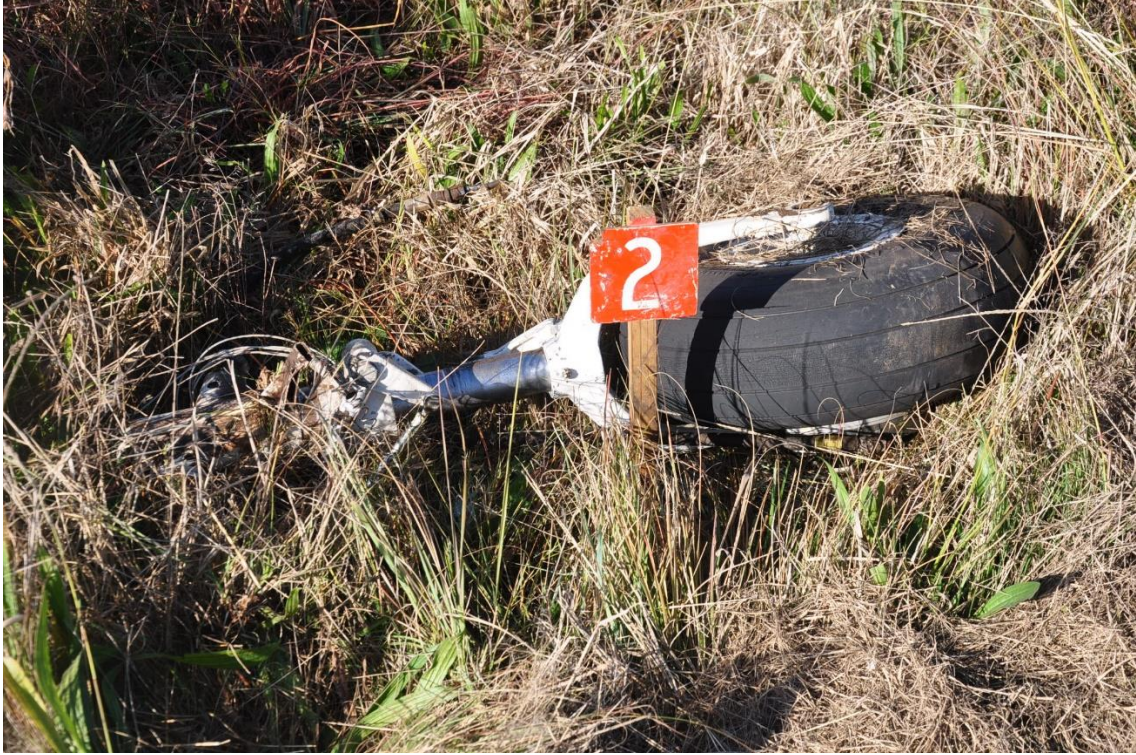
Figure 5: The main undercarriage strut and wheel that broke off.
