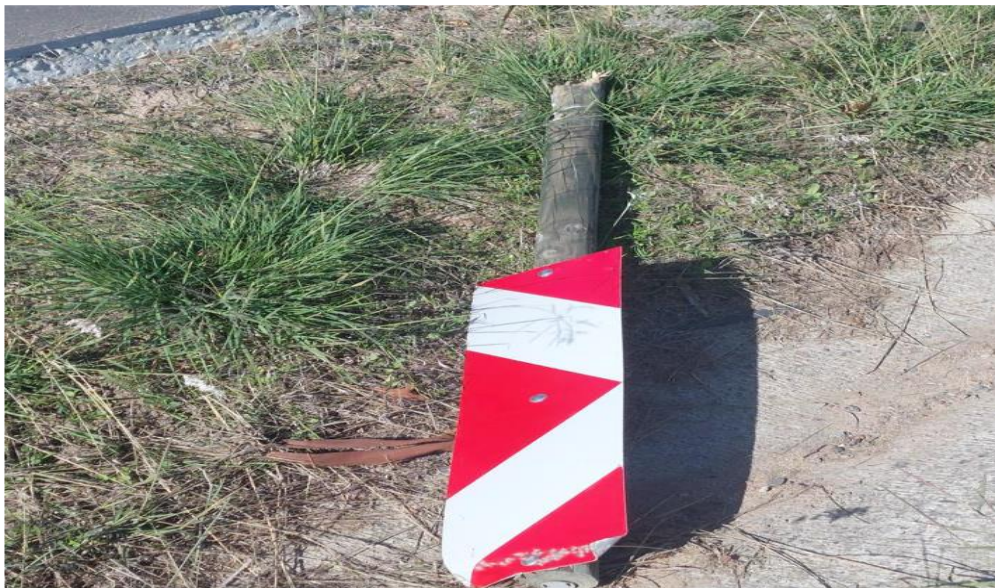
Figure 3: The severed road traffic sign pole.
