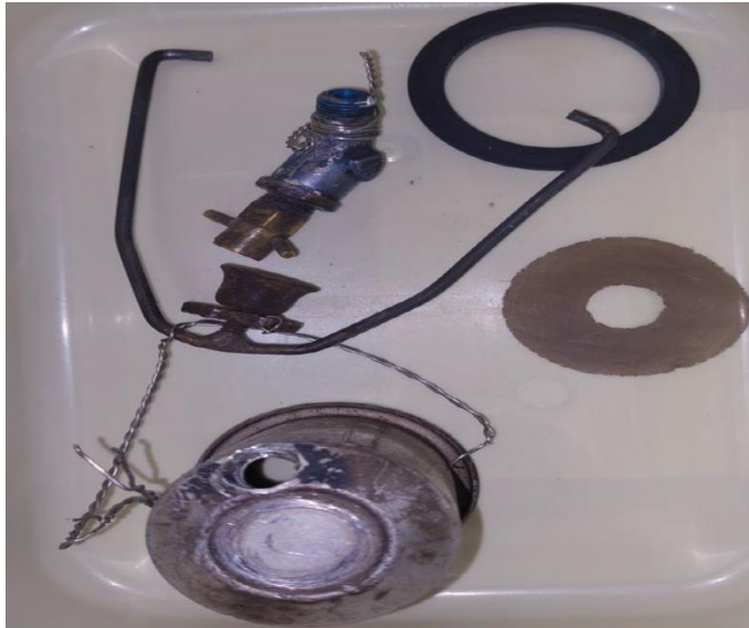
Figure 6: The damaged gascolator.
