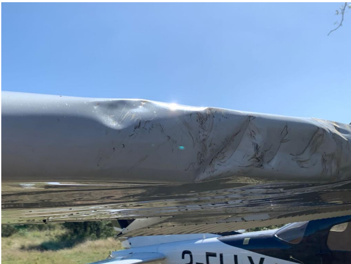
Figure 5: Damage to the right-side wing leading edge outboard. (Source: Owner)
