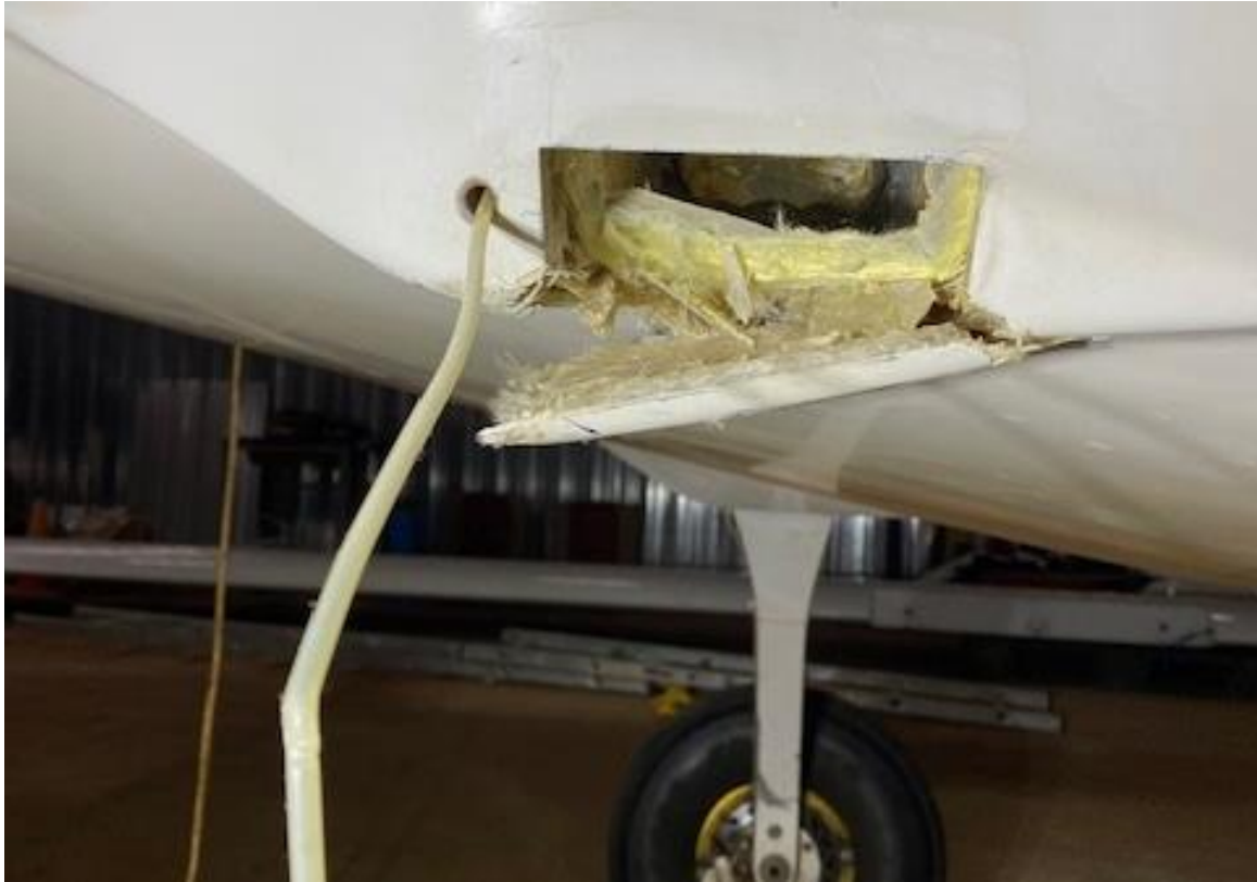
Figure 4: Damage caused to the fuselage where the right main gear strut was fitted. (Source: Pilot)
