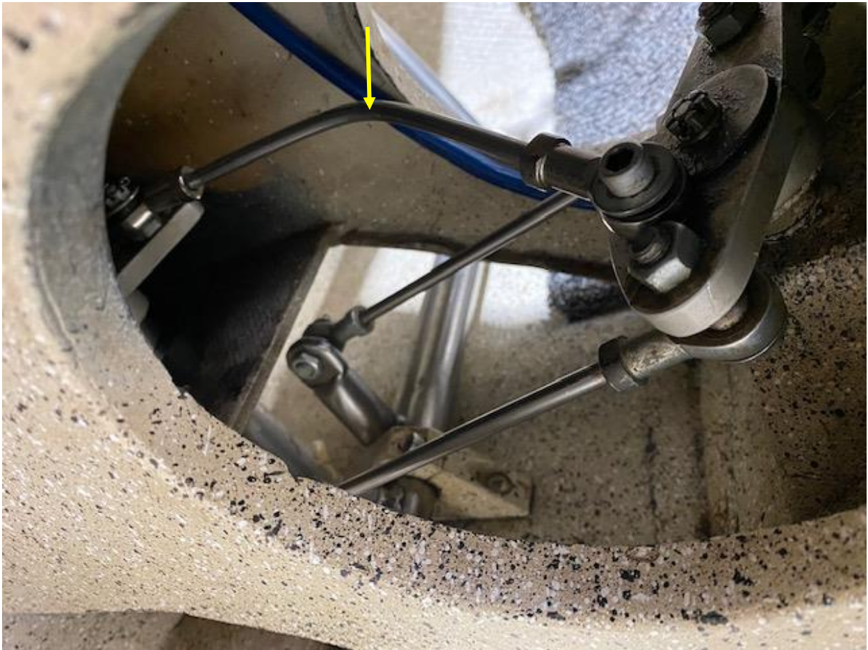
Figure 5: The yellow arrow indicates the bend in the nose gear steering rod. (Source: Pilot)
