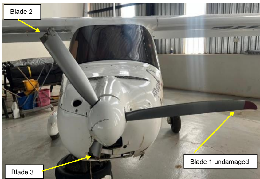
Figure 4: The propeller blades post-accident.
