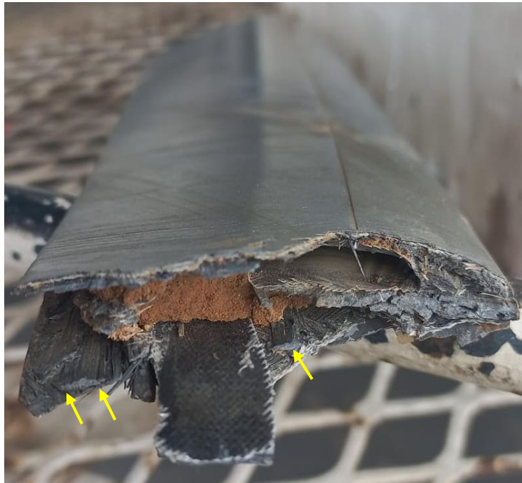
Figure 6: An enlarged blade number 3 tip showing carbon fibre layers.
