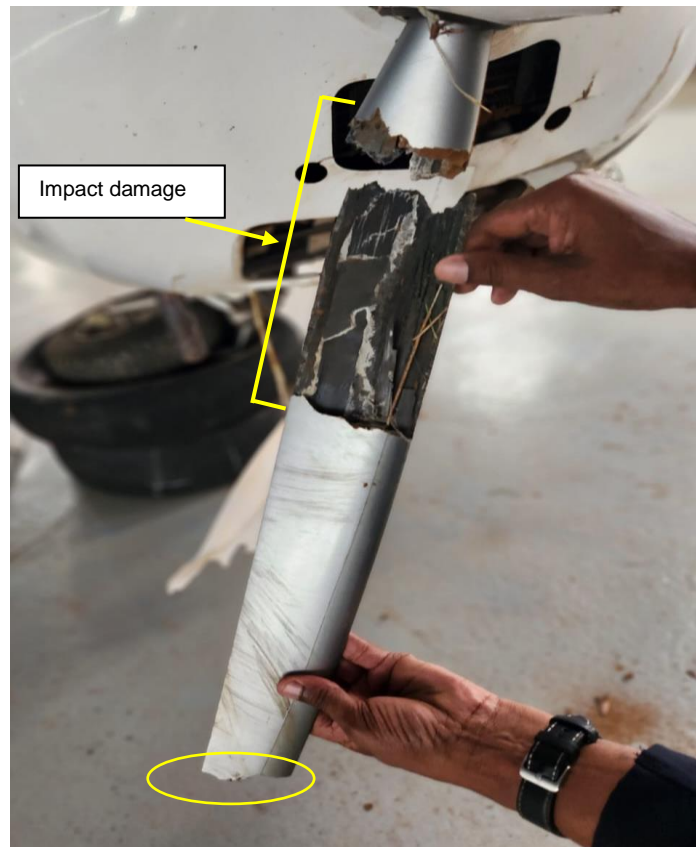
Figure 5: Reconstructed blade number 3 showing damage sustained on the cord and the tip that had fractured.
