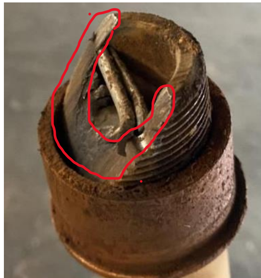
Figures 2 and 3: The sheared castellated nut (left) and the nose gear strut bottom area with a split pin. (Source: Operator)
