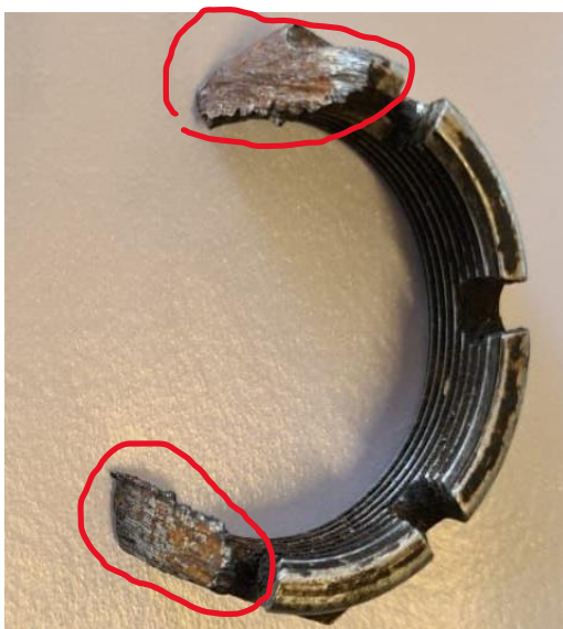
Figures 2 and 3: The sheared castellated nut (left) and the nose gear strut bottom area with a split pin. (Source: Operator)
