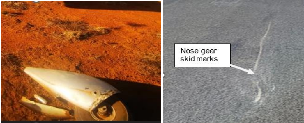
Figures 5 and 6: The separated lower end part of the nose gear (left) and the skid marks on the runway surface (right). (Source: Operator)
