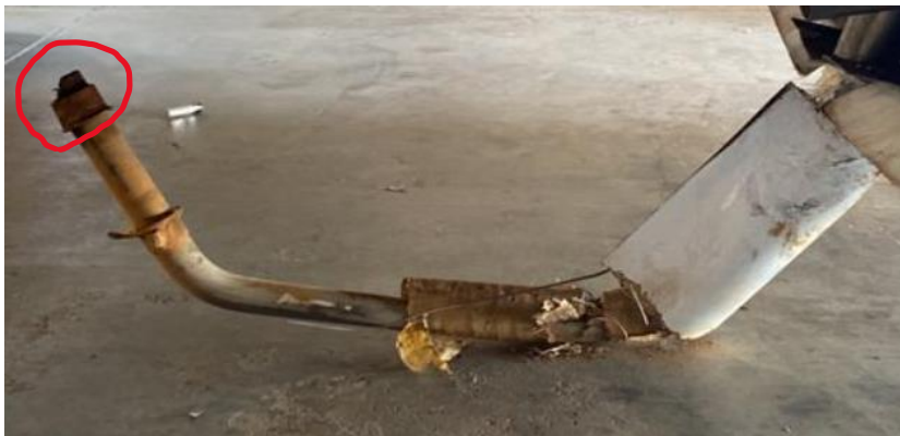
Figure 4: The nose gear strut that bent backward. (Source: Operator)
