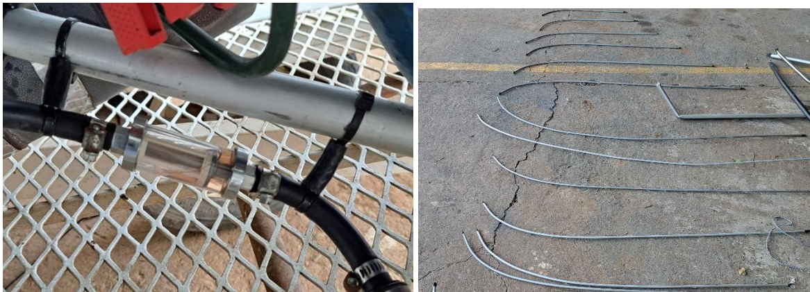
Figure 3 and 4: Fuel filter with some fuel and vacuum (left), and bent wing ribs (right).
