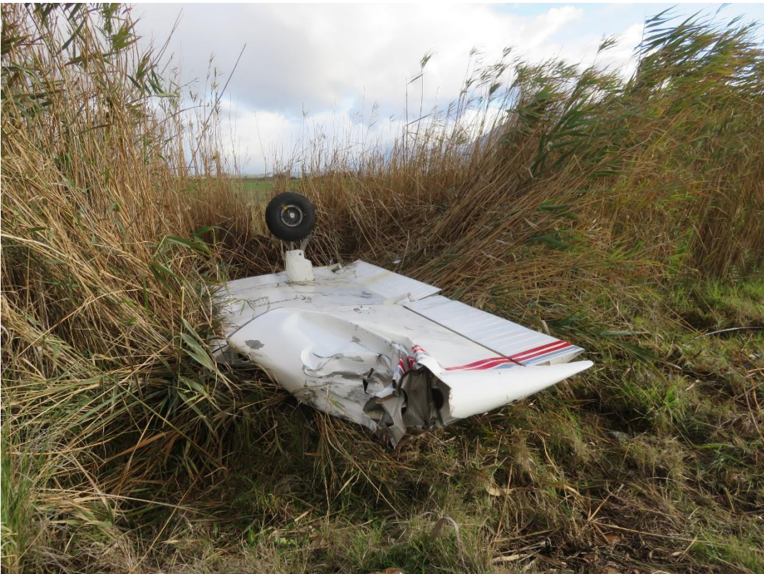
Figure 8: The right wing which was ripped off from the fuselage.
