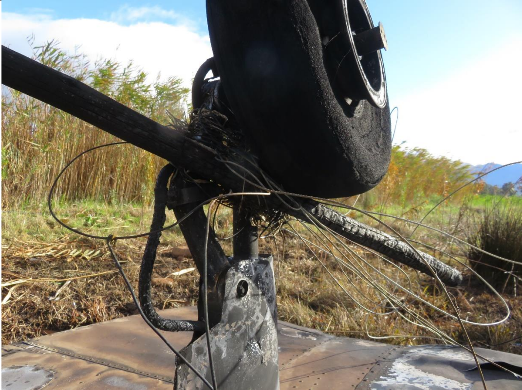
Figure 7: The left main gear with the barbed wire wrapped around it.
