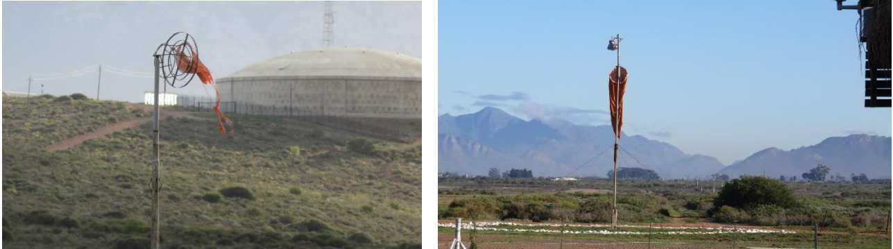
Figure 12: The dilapidated windsock (left side), and the primary windsock (right side). These photographs were taken during the on-site investigation.
