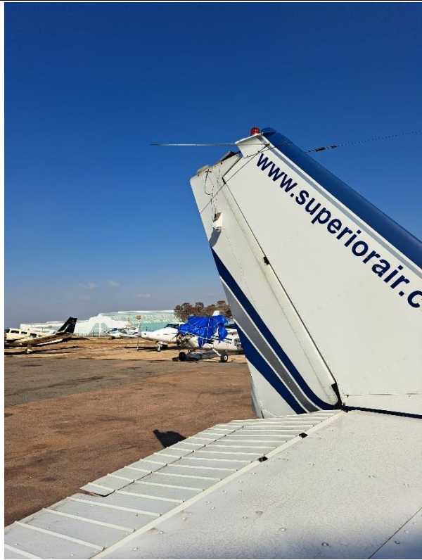
Figures 2 and 3: The damaged propeller blade (left) and the rudder without the counterweight that got separated (right).
