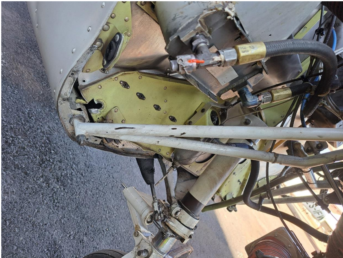
Figure 4: The damaged firewall and the deflated oleo.
