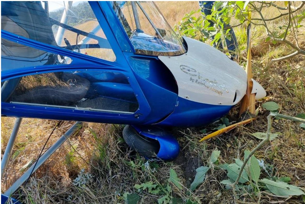
Figure 2: The damage sustained by the aircraft. (Source: Pilot)
