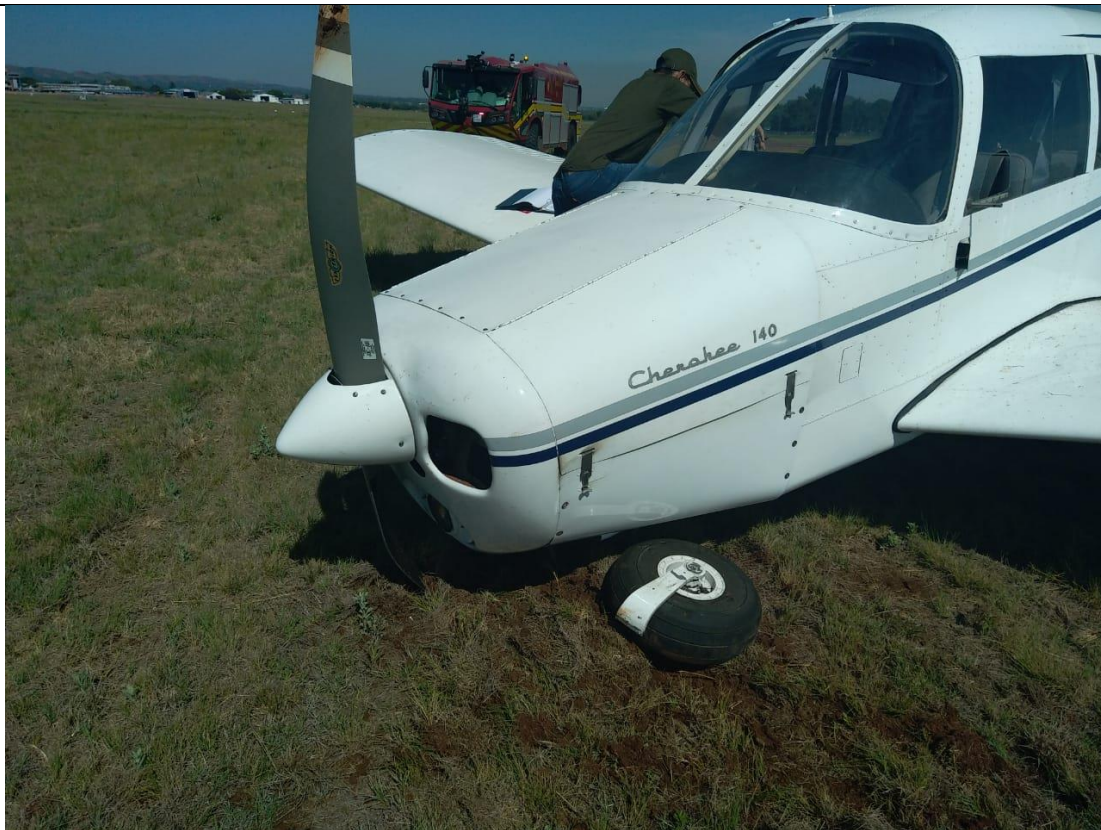
Figure 2: The broken nose wheel and the bent propeller blades. (Source: ATO)
