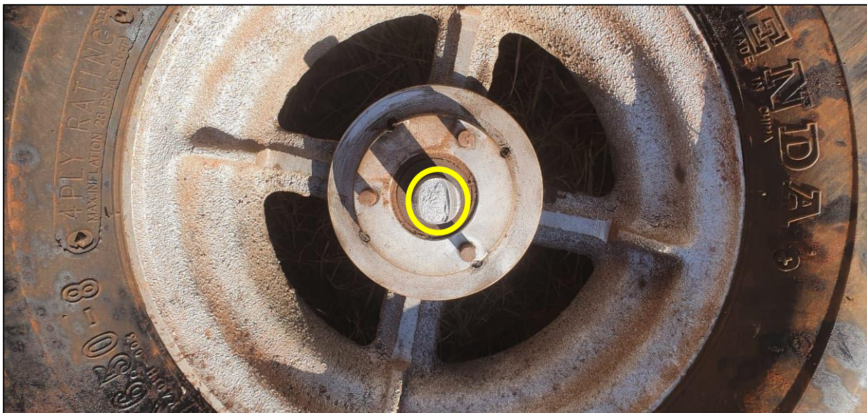
Figure 2: Location of the right axle fracture (in the yellow circle). (Source: Owner)
